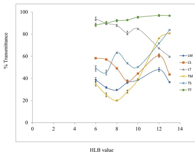
Fig. 1. The percent transmittance of the different emulsions prepared using different surfactant/cosurfactant mixtures at different HLB values.
