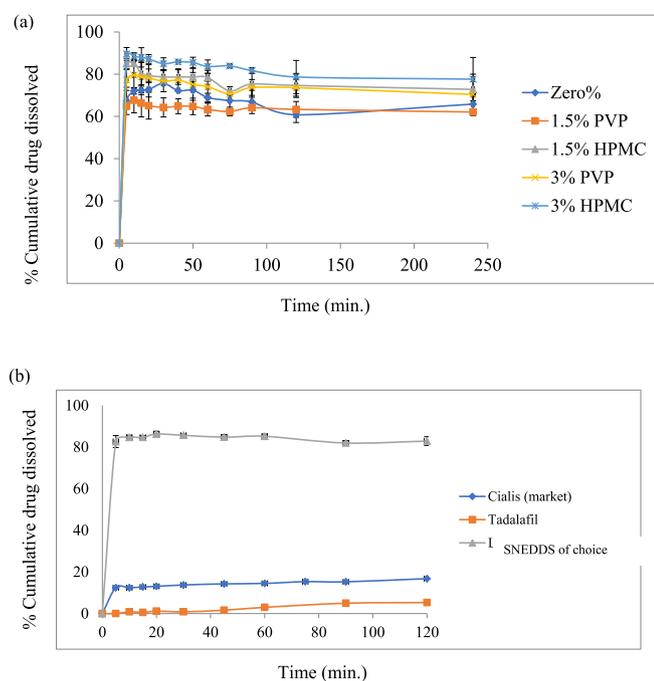
**Fig. 5.** (a) *In-vitro* precipitation test of tadalafil from the different formulae. (b) *In-vitro* dissolution profiles of pure drug tadalafil, market product and selected SNEDDS formula.
