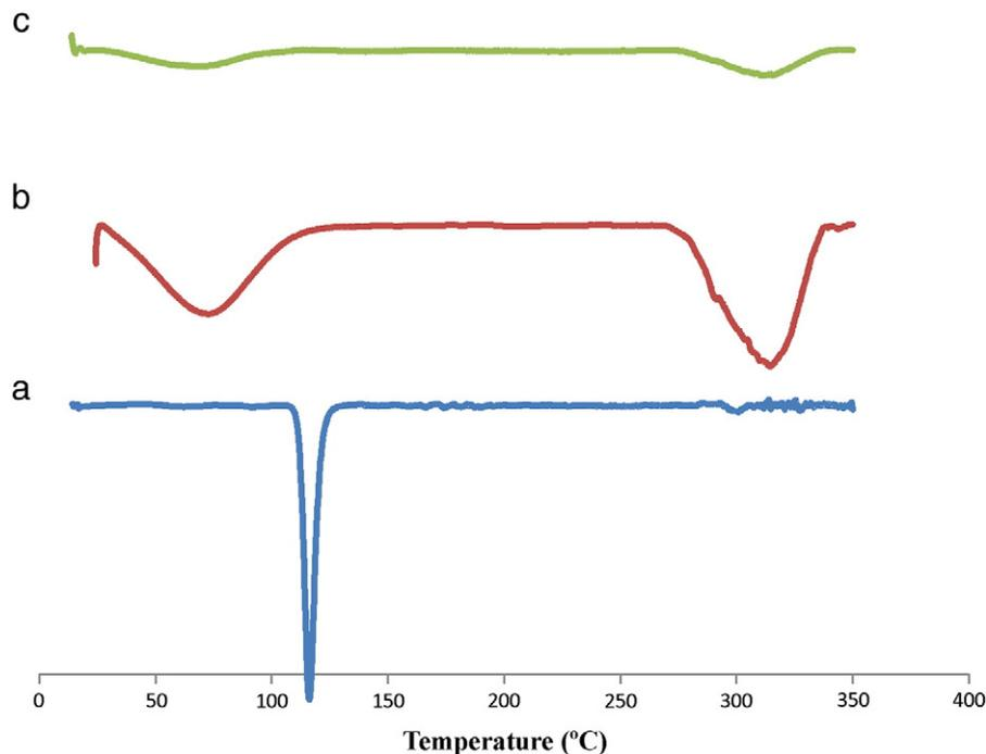
Fig. 4. DSC thermograms of CAR plain powder (a), Soluplus® (b) and CAR in the selected freeze-dried solid dispersion formulation (c).
