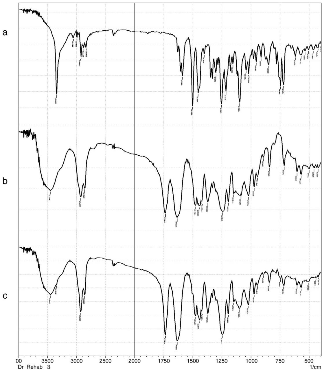
Fig. 6. FT-IR spectra of CAR plain powder (a), Soluplus® (b) and CAR in the selected freeze-dried solid dispersion formulation (c).
