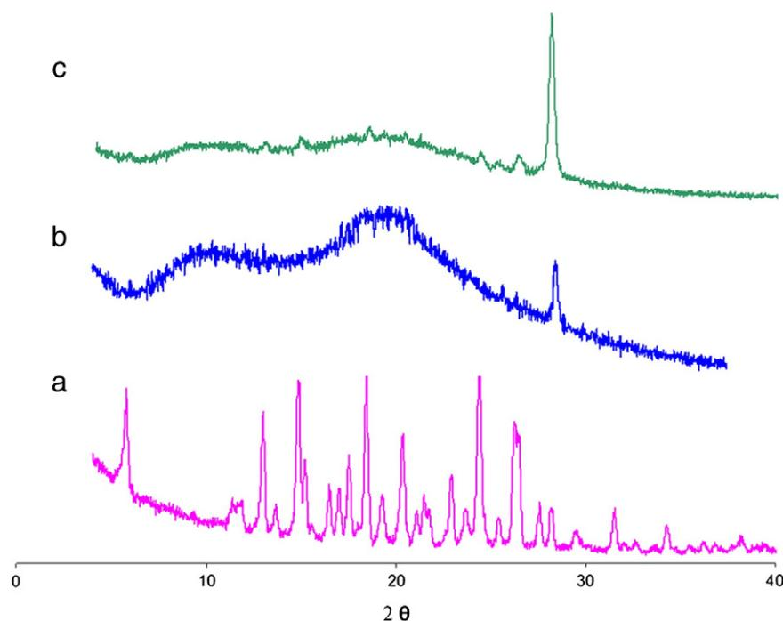
Fig. 5. X-ray diffractograms of CAR plain powder (a), Soluplus® (b) and CAR in the selected freeze-dried solid dispersion formulation (c).
