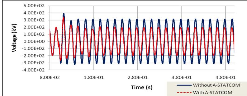
Figure 9. Mitigation of 312.436 (kV) [1.6 (p.u.)] voltage swell using Advanced STATCOM for IEEE 118 bus system
