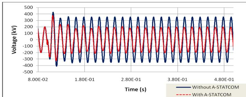
Figure 11. Mitigation of 351.54 (kV) [1.8 (p.u.)] voltage swell using Advanced STATCOM for IEEE 118 bus system
