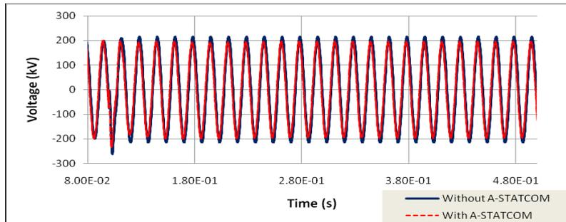
Figure 4. Mitigation of 214.7944 (kV) [1.1 (p.u.)] voltage swell using Advanced STATCOM for IEEE 118 bus system
