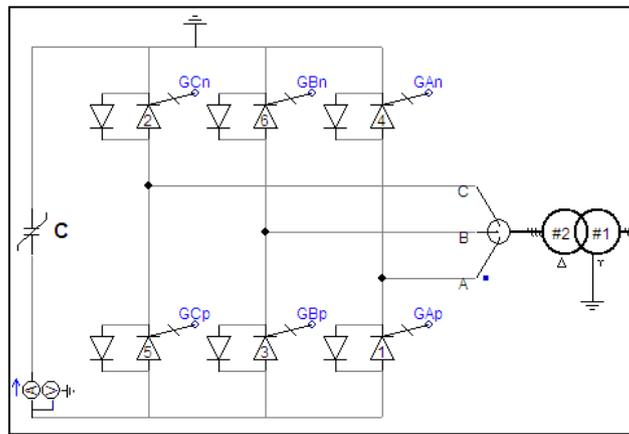
Figure 1. Structure of Advanced STATCOM implemented in PSCAD/EMTDC program
