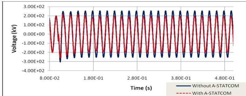
Figure 6. Mitigation of 253.948 (kV) [1.3 (p.u.)] voltage swell using Advanced STATCOM for IEEE 118 bus system
