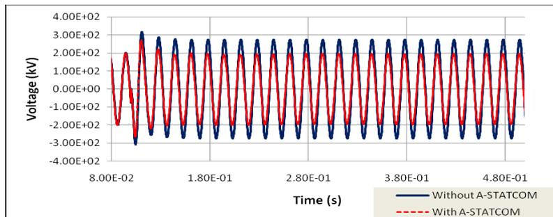
Figure 7. Mitigation of 273.524 (kV) [1.4 (p.u.)] voltage swell using Advanced STATCOM for IEEE 118 bus system
