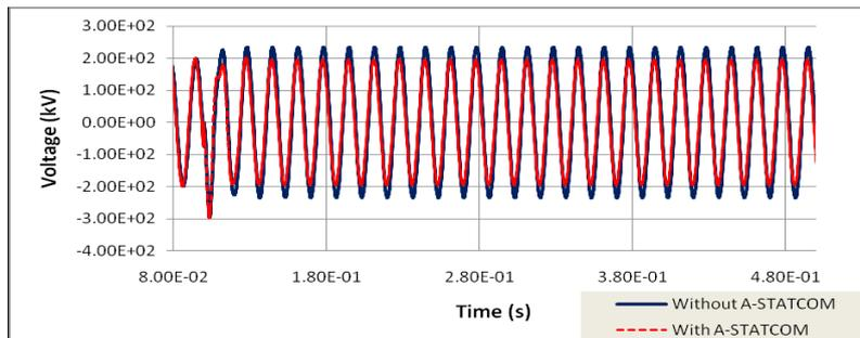
Figure 5. Mitigation of 234.504 (kV) [1.2 (p.u.)] voltage swell using Advanced STATCOM for IEEE 118 bus system
