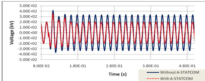
Figure 10. Mitigation of 331.803 (kV) [1.7 (p.u.)] voltage swell using Advanced STATCOM for IEEE 118 bus system
