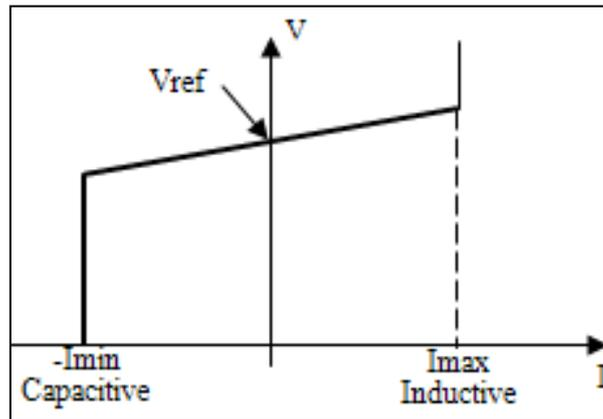
Figure 2. STATCOM V-I characteristics curve for different operating condition
