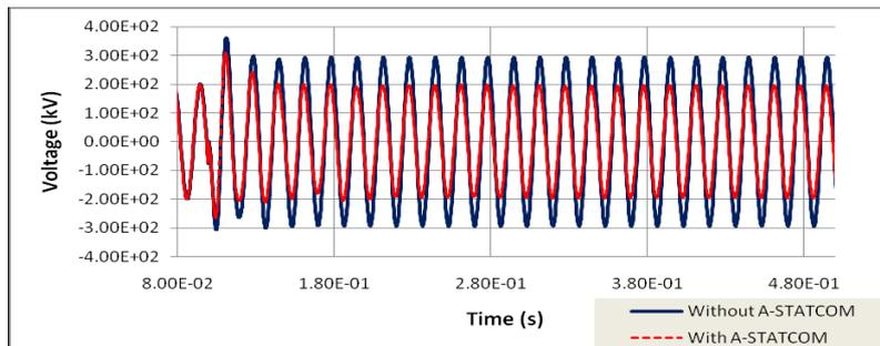
Figure 8. Mitigation of 292.991 (kV) [1.5 (p.u.)] voltage swell using Advanced STATCOM for IEEE 118 bus system
