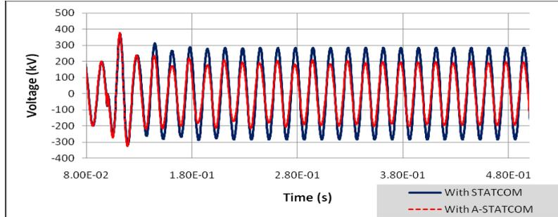
Figure 3. Comparison between traditional STATCOM and Advanced STATCOM (A-STATCOM) to mitigate 1.8 p.u. swell for IEEE 118 bus system
