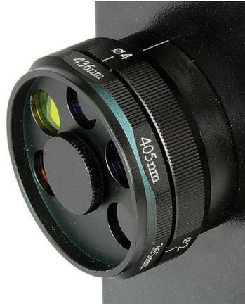
Figure 2: filter wheel and aperture selection ring
