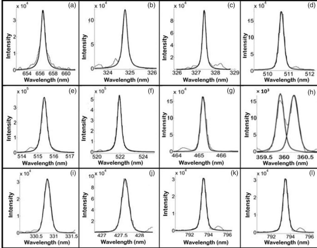
**Figure 2.** (a–l) Emission spectral lines of neutral copper at arbitrary delay of  $4 \mu\text{s}$ , gate of  $1 \mu\text{s}$ , and together with best fitting to Voigt function (thick solid lines).
