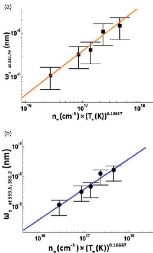
**Figure 6.** Variation of the estimated Stark broadening parameters of the (a) Cu(I) line at 330.79 nm and (b) the two lines at 359.91, 360.2 nm with plasma parameters (density and temperature).
