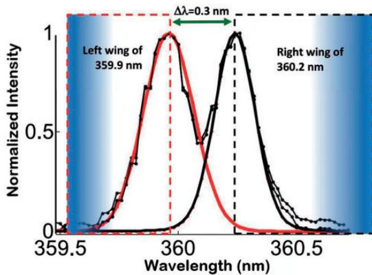
**Figure 4.** Voigt fitting (red curve at 359.9 nm and black curve at 360.2 nm) to spectral line data (black dotted curve) showing the wings (dashed squares) used to evaluate electron density from both lines at wavelengths 359.91 (unhighlighted left) and 360.2 nm (unhighlighted right) at arbitrary delay time of 5  $\mu$ s.
