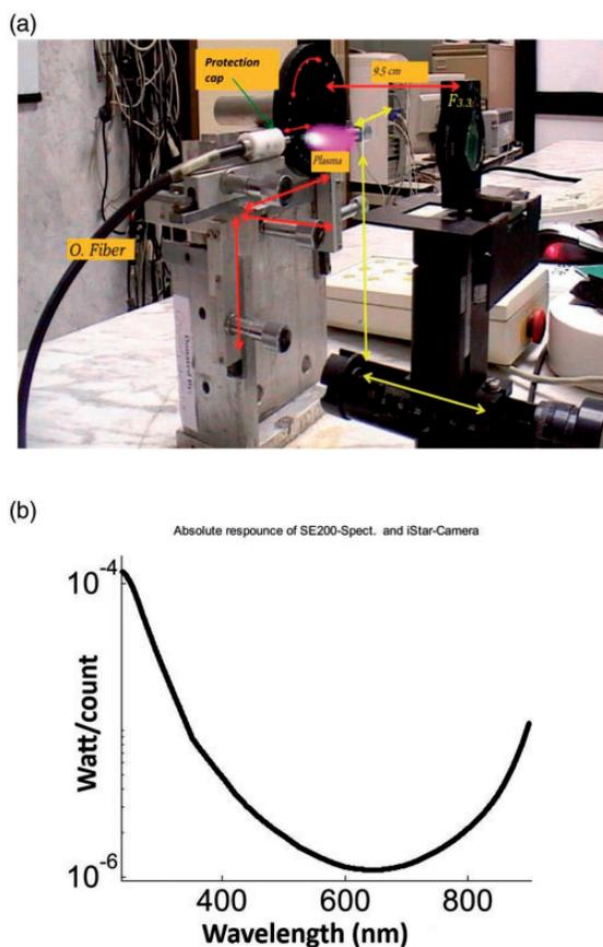
**Figure 1.** (a) A photograph of the homemade  $x,y,\phi$  target holder and (b) the absolute spectral sensitivity of the measuring apparatus including optical fiber, SE200 spectrograph, and the ICCD camera.
