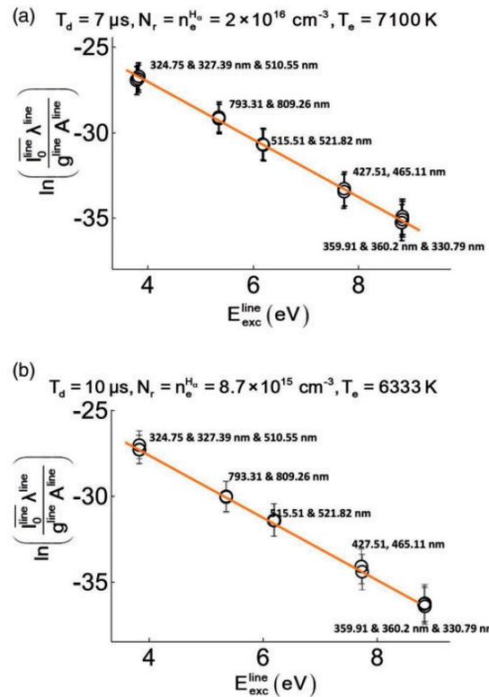
**Figure 5.** Boltzmann plots at different delay times (a) 7  $\mu$ s and (b) 10  $\mu$ s with values corresponding to three Cu(I) transition lines (at the far right side of the graph) coincide with linear plot.
