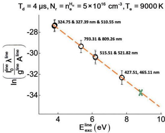
**Figure 3.** Boltzmann plot constructed at delay time 4  $\mu$ s using nine well-known transition probabilities and Stark broadening parameters of Cu(I) lines at 324.75, 327.39, 427.51, 465.11, 510.55, 515.32, 521.82, 793.31, and 809.26 nm (open circles) with green cross indicating the appropriate location of the unknown Stark broadening parameters of transition at 330.79, 359.91, and 360.2 nm.
