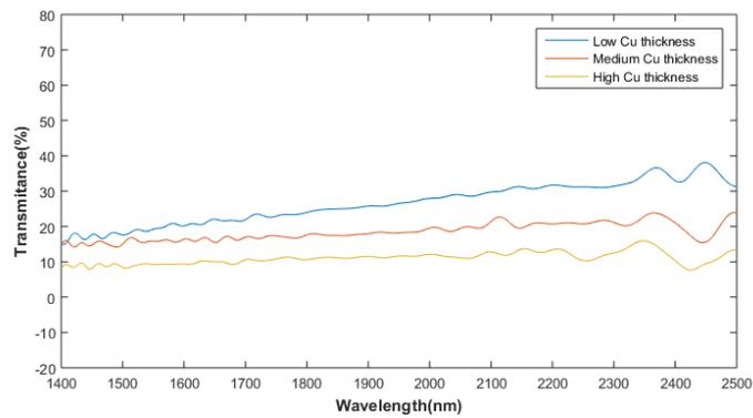
Figure 7. Cu coated BSi reflection measurement
