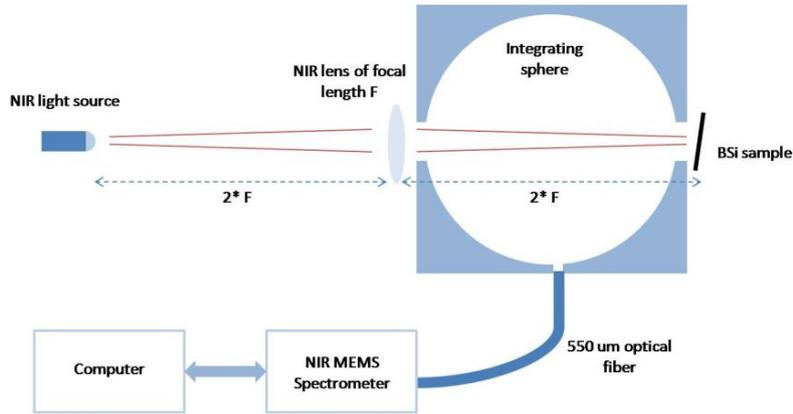
Figure 5. Transmission measurement setup
