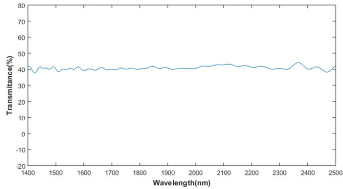
Figure 6. Bare BSi transmission measurement
