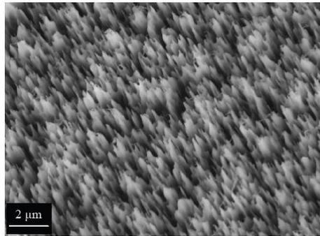
Figure 1. An SEM of the surface of the fabricated black silicon
