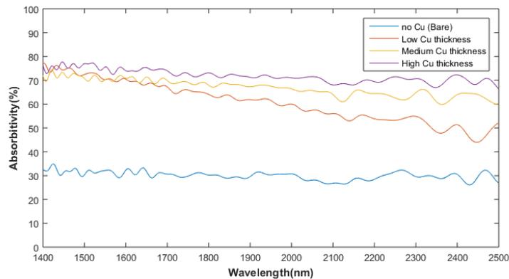
Figure 8. Absorptivity of bare and Cu coated BSi
