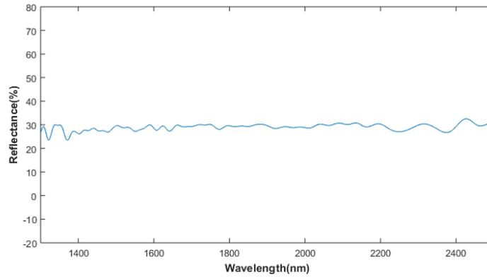
Figure 3. Bare BSi reflection measurement
