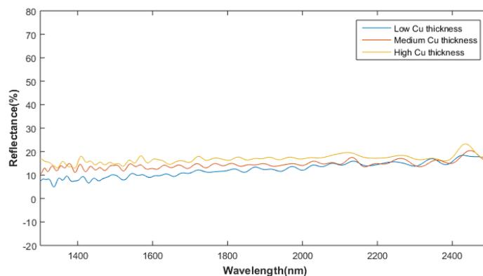
Figure 4. Cu coated BSi reflection measurement
