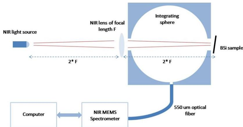
Figure 2. Reflection measurement setup
