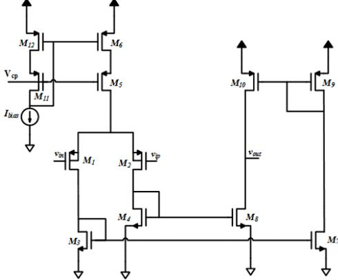
Fig. 6 Main OTA Circuit Schematic [7]
