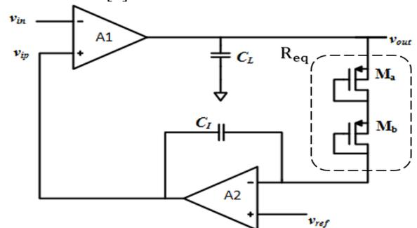
Fig. 5 LNA with the active feedback network Circuit Schematic [7]
