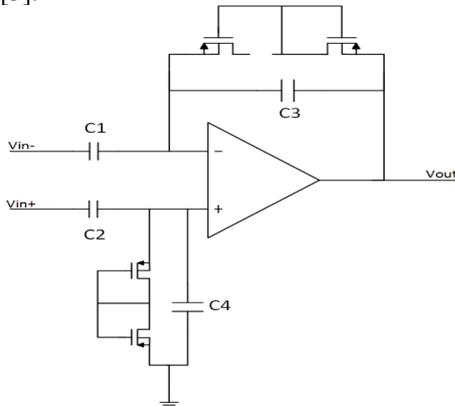
Fig. 3 Single Ended pre-amplifier Schematic [3]
