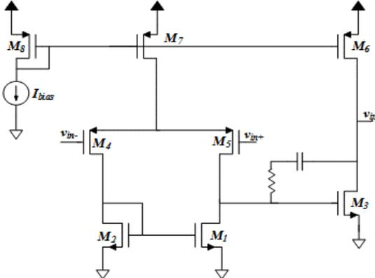
Fig. 7 Feedback OTA Circuit Schematic [7]
