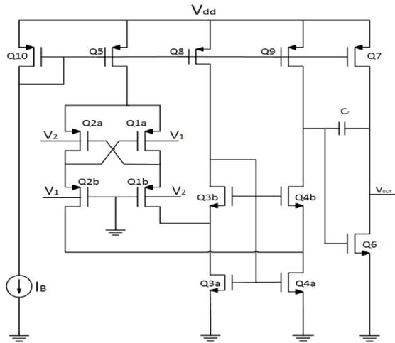
Fig. 9 Optimized Bulk-Driven OTA Circuit Schematic [10]
