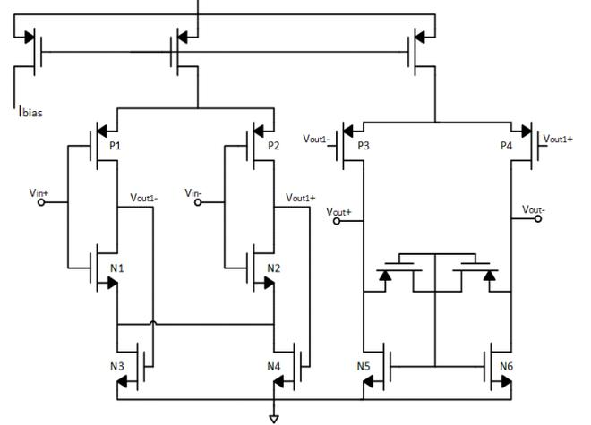
Fig. 8 Fully Differential Current-Reuse OTA Circuit Schematic [11]
