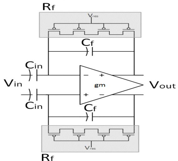
Fig. 1 Closed Loop LNA Schematic [4]
