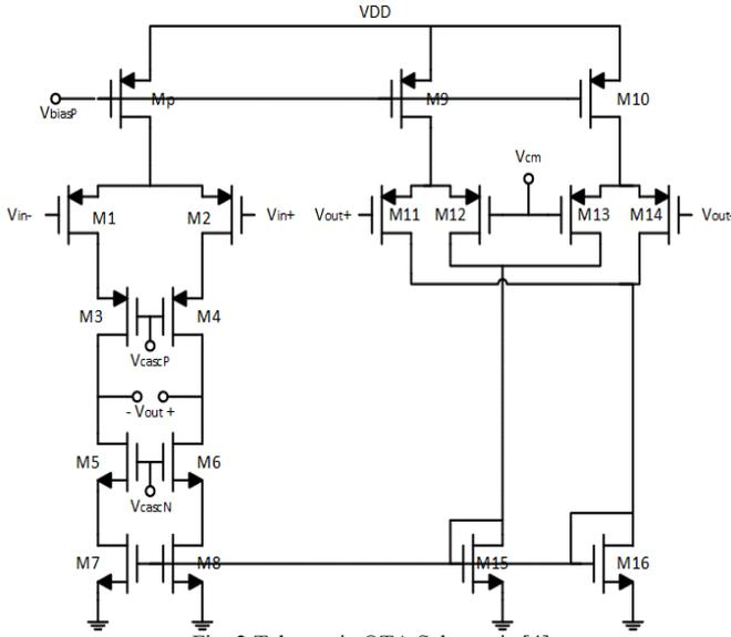
Fig. 2 Telescopic OTA Schematic [4]
