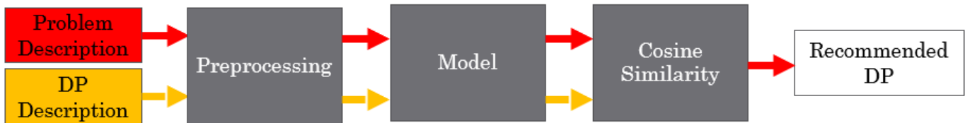
Fig. 2. Design pattern recommendation approach - Design pattern level
