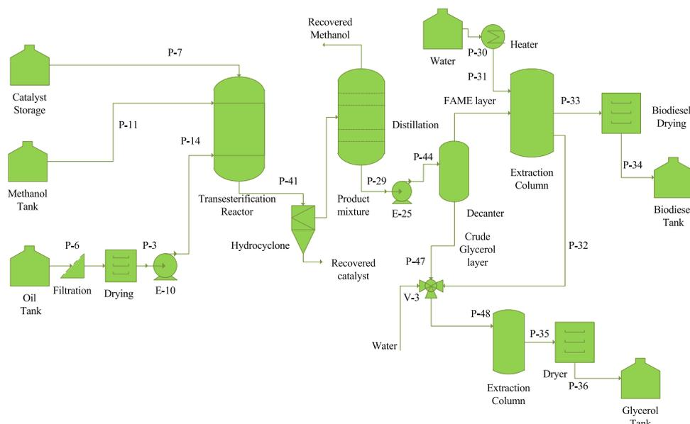
Fig. 1. Schematic diagram of algal biofuel production processes catalyzed by  $\text{Na}_4\text{SiO}_4$ .
