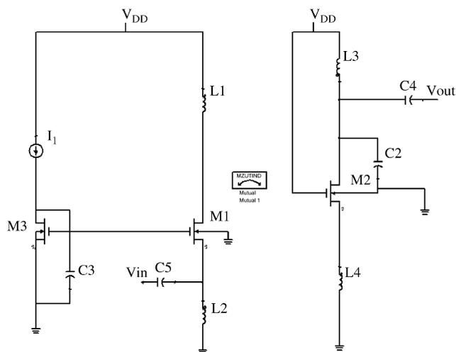
Fig. 2. Modified cascade low-noise amplifier.
