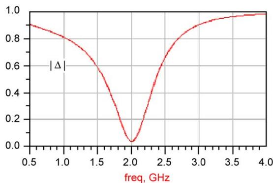
Fig. 4. Stability condition (5) and stability factor  $K$ .
