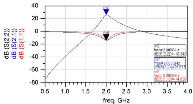
Fig. 3. Input return loss, gain, and output return loss of the LNA.
