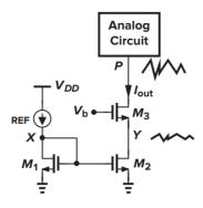
$$I_{out} = I_{D2} = I_{REF} \times \frac{1 + \lambda V_{DS2}}{1 + \lambda V_{DS1}} = I_{REF} \times \frac{1 + \lambda (V_{GS1} + \Delta V_y)}{1 + \lambda V_{GS1}}$$
