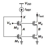
$$\begin{split} I_{out} &= I_{D3} = 3I_{REF} \times \frac{1 + \lambda V_{DS3}}{1 + \lambda V_{DS1}} = 3I_{REF} \times \frac{1 + \lambda (V_{ov1} + \Delta V_B)}{1 + \lambda V_{ov1}} \qquad (I) \\ I_{out} &= I_{D4} = \frac{1}{2} K_{n4} (V_{GS4} - V_{TH})^2 (1 + \lambda V_{DS4}) = \frac{1}{2} K_{n4} (V_{GS2} - \Delta V_B - V_{TH})^2 (1 + \lambda (V_{TH} + 1 - \Delta V_B)) \quad (II) \end{split}$$
