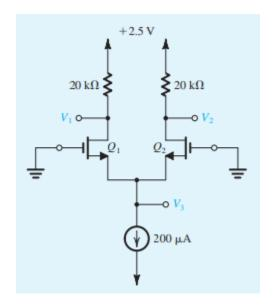
**Problem 1.8:** For the circuits shown below, assume  $\mu$ nCox =  $3\mu$ pCox =  $270 \mu$ A/V2, |Vt|=0.5V,  $\lambda$  = 0, L = 1  $\mu$ m, and W = 3  $\mu$ m, unless otherwise specified. Find the labeled currents and voltages.
