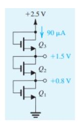
**Problem 1.7:** 1 In the circuit shown on the right, transistors Q1 and Q2 have Vt = 0.7 V, and the process transconductance parameter  $\mu$ nCox =125  $\mu$ A/V2. Find V1, V2, and V3 for each of the following cases:
