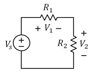
$$V_1 = \frac{R_1}{R_1 + R_2} \times V_S$$
