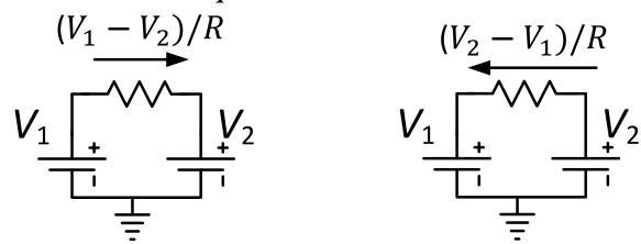
• Solve the resulting simultaneous equations to obtain the unknown node voltages.
