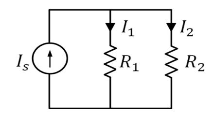
$$I_1 = \frac{R_2}{R_1 + R_2} \times I_S$$
