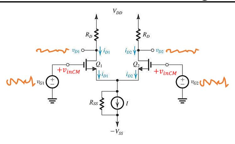
$$v_{D1} = v_{D2} = -\frac{g_m R_D v_{inCM}}{1 + 2g_m R_{SS}} \approx -\frac{R_D}{2R_{SS}} v_{inCM} (if \ 2g_m R_{SS} \gg 1)$$
