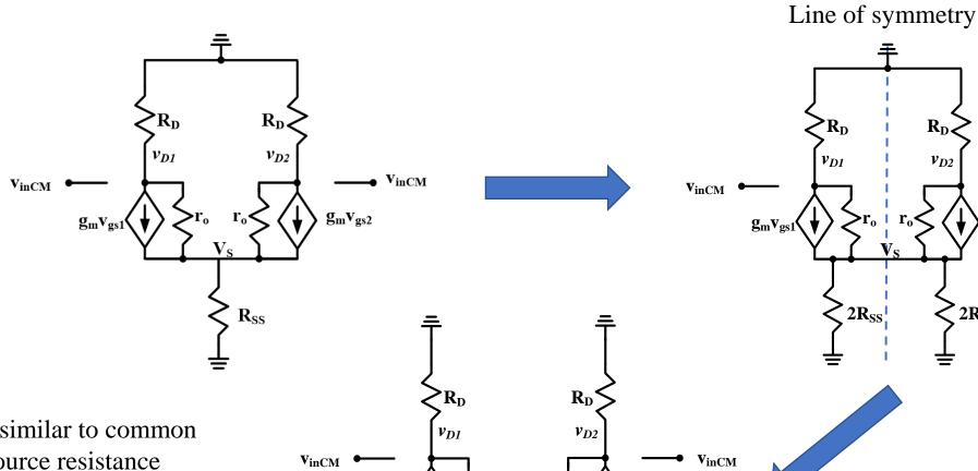
The circuit is similar to common source with source resistance
