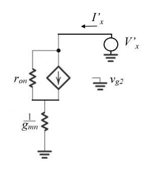
$$R_3 = r_{on} + R_2 + g_{mn}r_{on}R_2 \approx 2r_{on}$$
