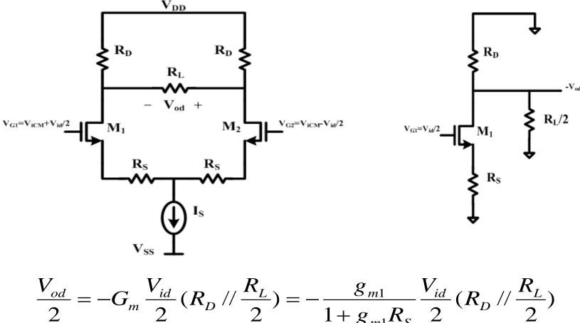
$$\frac{\mathbf{v}_{od}}{2} = -G_{m} \frac{\mathbf{v}_{id}}{2} (R_{D} / / \frac{R_{L}}{2}) = -\frac{g_{m1}}{1 + g_{m1} R_{S}} \frac{\mathbf{v}_{id}}{2} (R_{D} / / \frac{R_{L}}{2})$$
