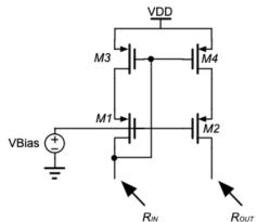
**Problem (3):** For amplifier shown below, assume  $\lambda = 0$  and all devices are identical and in saturation.  $V_{th} = 1V$ , and  $V_{BIAS} = 2.5V$ .
