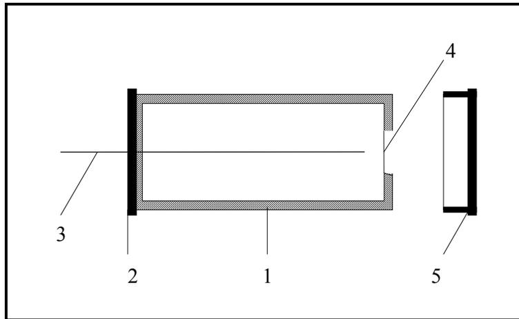
Figure (3): the Counter tube.
