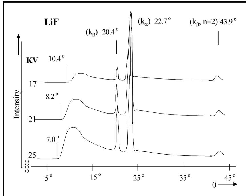
Figure (11): X-ray spectra produced at different high tension voltages.
