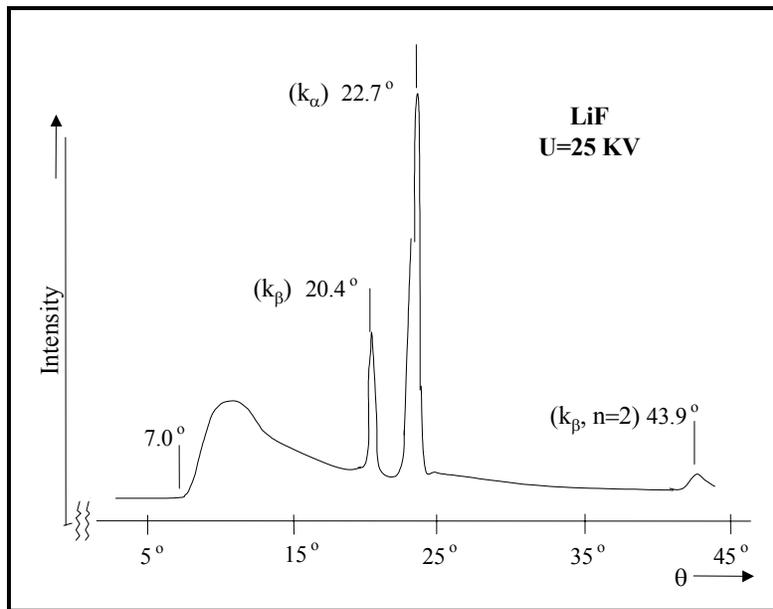
Figure (8): X-ray spectrum scattered from LiF monocrystal.
