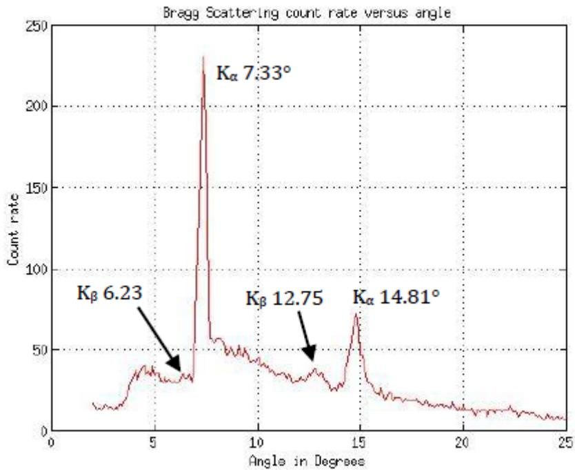
Figure (9): X-ray spectrum scattered from NaCl monocrystal.
