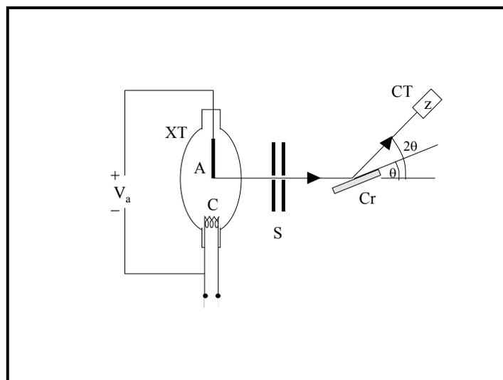
Figure (2): Diagrammatic representation of the arrangement used for Bragg reflection ( $V_a$  = anode voltage, XT = X-ray tube, C = cathode, A = copper anticathode, S = screen system, Cr = crystal, CT = Counting tube,  $\theta$  = Bragg angle).
