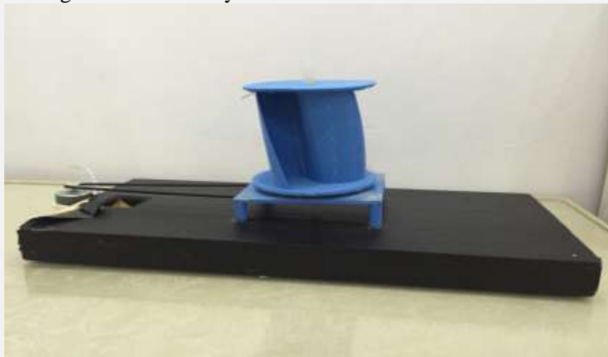
Figure 8: Assembly of the miniature Savonius VAWT with the generator.
