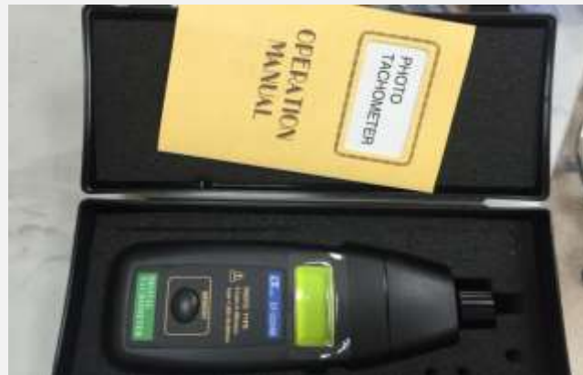
Figure 6: Tachometer used for measuring the blades rotational speed.
