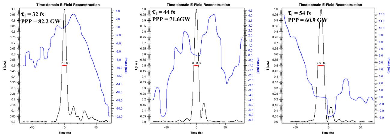
**Fig. 4.** The temporal profile change of the output pulses  $\tau_i$  values of 32, 44, and 54 fs, respectively, at neon gas pressure of 2.25 atm. The compressed output pulse (black curve) and temporal phase (blue curve) of the compressed output pulses were measured using SPIDER. (For interpretation of the references to color in this figure legend, the reader is referred to the web version of this article.)
