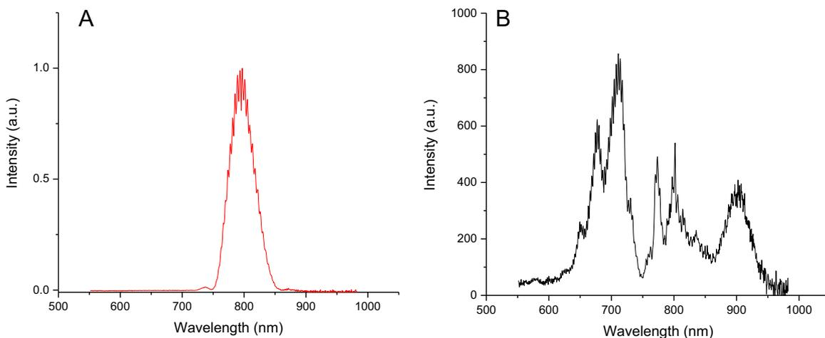
**Fig. 2.** (A) The 46 nm bandwidth of the Ti:sapphire oscillator at 795.3 nm and 18 fs pulse duration. (B) The 350 nm broadband width of the output pulses of 7 fs and energy of 600  $\mu$ J.
