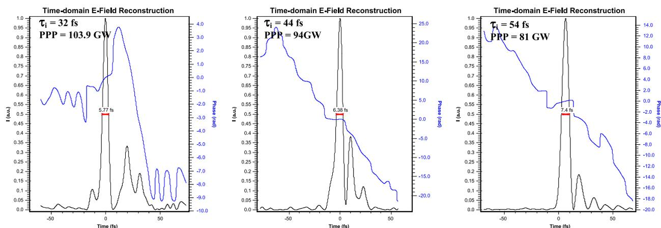
**Fig. 5.** The temporal profile change of the output pulses  $\tau_i$  values of 32, 44, and 54 fs, respectively, at neon gas pressure of 2.5 atm. The compressed output pulse (black curve) and temporal phase (blue curve) of the compressed output pulses were measured using SPIDER. (For interpretation of the references to color in this figure legend, the reader is referred to the web version of this article.)
