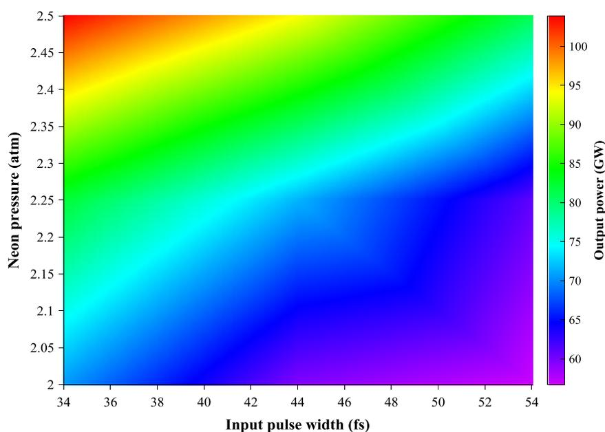
**Fig. 6.** A summarized 2D contour representation of time-domain electric field reconstructed pulse profile of the observed TLPPP values from 56.7 to 103.9 GW for different  $\tau_i$  values in the range from 32 to 54 fs, and neon gas pressures from 2 to 2.5 atm. (For interpretation of the references to color in this figure, the reader is referred to the web version of this article.)
