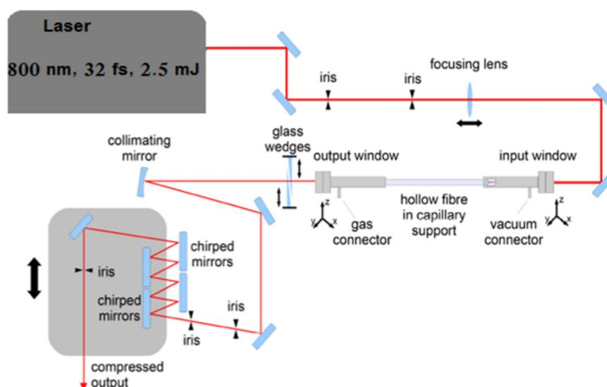
Fig. 1. Schematic of the ultrafast white-light radiation system with variable peak power.
