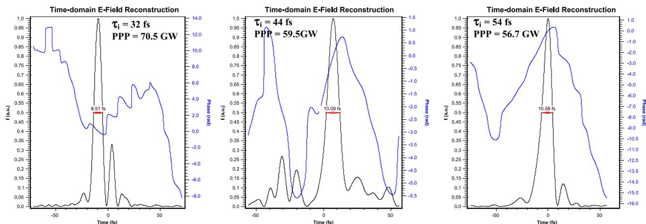
**Fig. 3.** The temporal profile change of the output pulses  $\tau_i$  values of 32, 44, and 54 fs, respectively, at neon gas pressure of 2 atm. The compressed output pulse (black curve) and temporal phase (blue curve) of the compressed output pulses were measured using SPIDER. (For interpretation of the references to color in this figure legend, the reader is referred to the web version of this article.)
