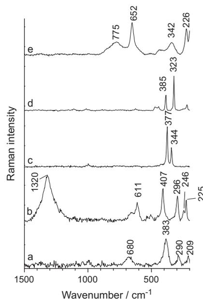
Fig. 3. Raman spectra (532 nm laser excitation) of iron minerals: (a) goethite, (b) hematite, (c) pyrite, (d) marcasite, and (e) pseudobrookite.
