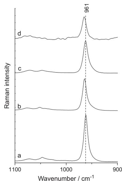
Fig. 5. FT-Raman spectra (1064 nm laser excitation) of (a) hydroxyapatite, (b) fluorapatite, (c) chlorapatite, and (d) phosphorite mineral.
