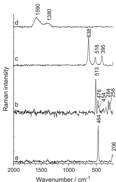
Fig. 4. Raman spectra (532 nm laser excitation) of (a) quartz, (b) microcline, (c) anatase, and (d) disordered carbon.
