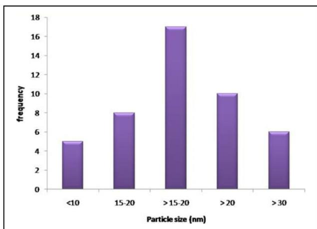
**Figure 2.** Number frequency histograms showing particle size distribution of ZnONPs in linear scale. The particle size data is based on the image analysis of more than 1000 particles. ZnONPs: zinc oxide nanoparticle.
