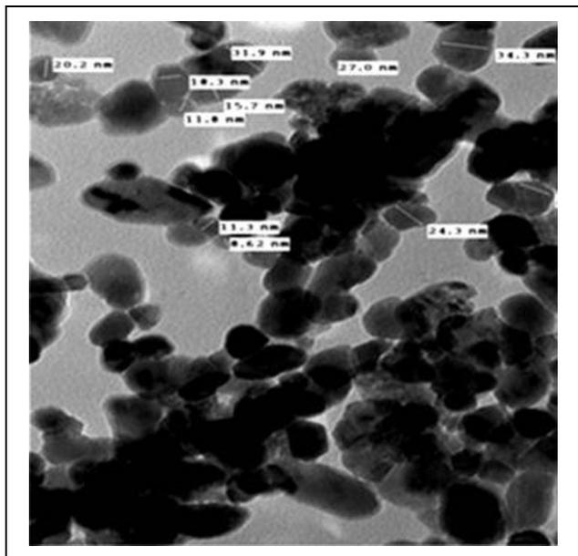
**Figure 1.** High-resolution TEM images of ZnONPs. TEM: transmission electron microscopic; ZnONPs: zinc oxide nanoparticle.
