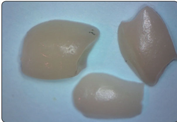
Fig. (6): Photographic representation of failure mode of Vita Suprinity crowns.
