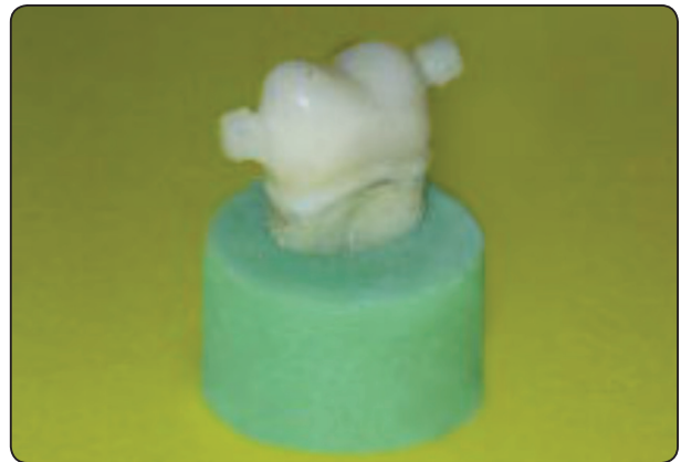
Fig (1) The cemented copings designed with cylindrical handles to facilitate pull-out testing.
