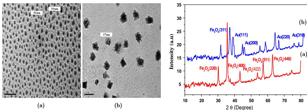
Fig. 1. TEM (left) images and XRD patterns of (right) (a) magnetic ( $\text{Fe}_3\text{O}_4$ ) nanoparticles, (b) gold-coated magnetic ( $\text{Au}@Fe_3\text{O}_4$ ) nanoparticles.<sup>15</sup>
