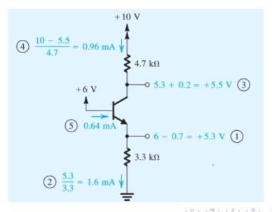
eta = 100Analyze this circuit to determine all node voltages and branch currents
