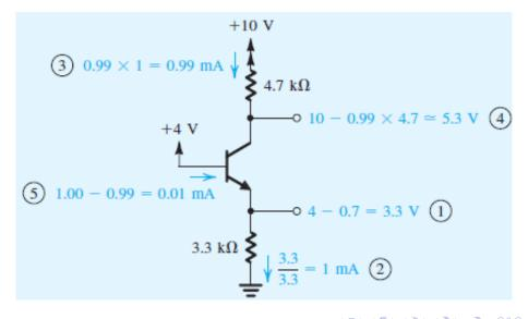
$\beta = 50$ Analyze this circuit to determine all node voltages and branch currents
