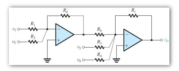
5- Find the relation between the output voltage and the input voltages. Assume ideal Op-Amps.
