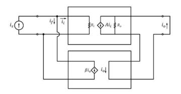
For the feedback to be negative,  $i_f$  must be of the **same** polarity as  $i_s$
