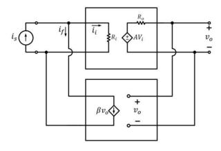
For the feedback to be negative,  $i_f$  must be of the **same** polarity as  $i_s$
