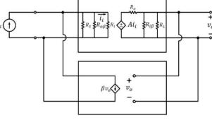
The finite source and load resistances also affect the values of A,  $R_i$ , and  $R_o$ .
