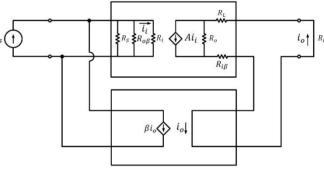
The finite source and load resistances also affect the values of A,  $R_i$ , and  $R_o$ .
