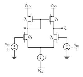
The capacitance  $C_m$  arises from  $C_{gs3}$ ,  $C_{gs4}$ ,  $C_{db3}$ ,  $C_{db1}$ , and the Miller effect of  $C_{gd1}$  and  $C_{gd4}$
