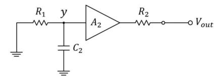
While calculating the pole at certain node, replace the capacitors at the other nodes by **open circuit**
