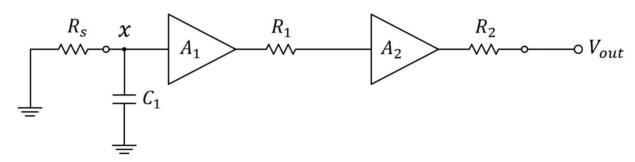
While calculating the pole at certain node, replace the capacitors at the other nodes by **open circuit**
