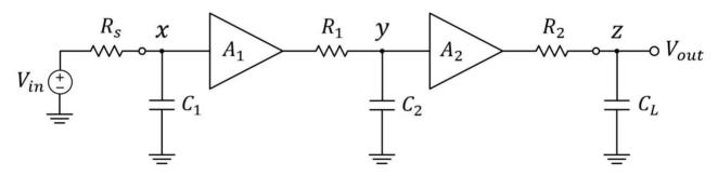
Each pole can be determine directly by calculating the reciprocal of the multiplication of the **total capacitance** seen from the node to **ground** by the **total resistance** seen from the node to **ground** after **shutting down** the input.
