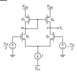
The common pole appears as a **single** pole in the total transfer function
