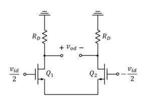
The frequency characteristics of the differential half circuit is **identical** to that of the common source amplifier
