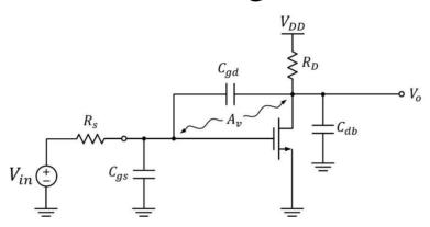
To simplify the analysis, Miller's **approximation** is used to convert  $C_{qd}$  in two grounded capacitors
