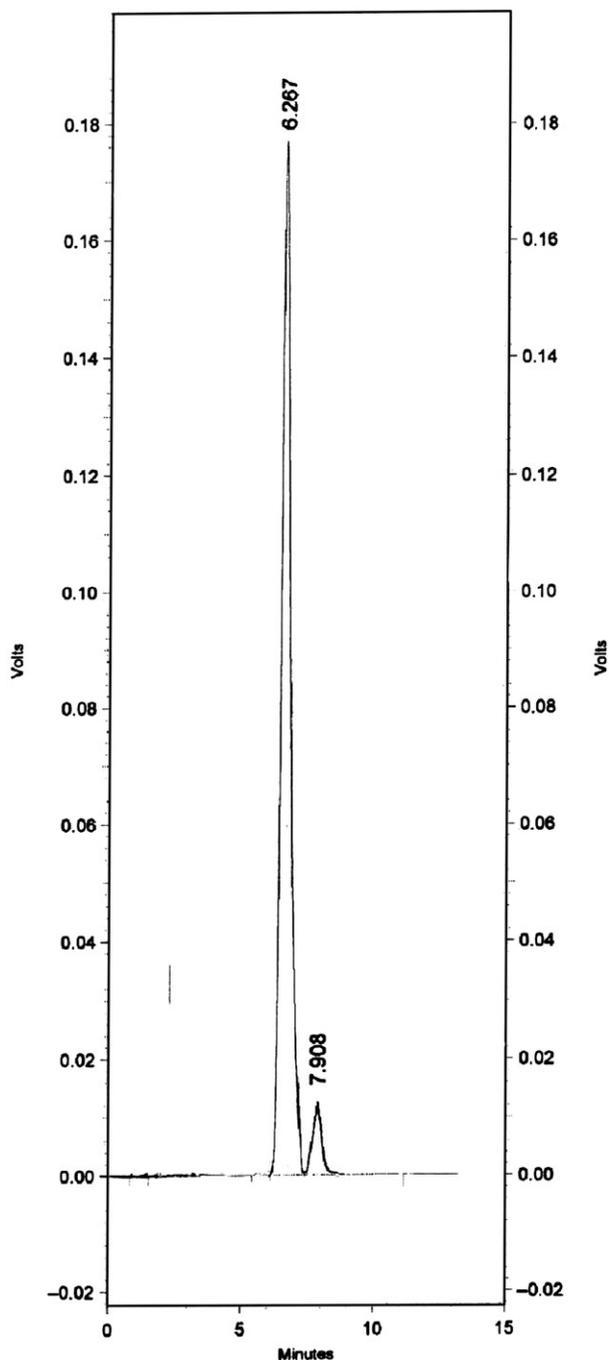
Figure 3. HPLC chromatogram for OMC (at 6.267 min) in the presence of its photodegradation (at 7.908 min).
