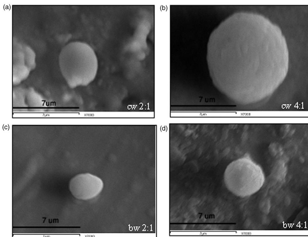
Figure 1. SEM images (magnification: 7000 $\times$ ) for the following polymer to drug ratios: (a) cw 2:1, (b) cw 4:1, (c) bw 2:1 and (d) bw 4:1.
