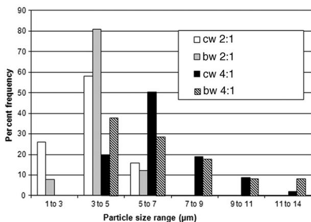
Figure 2. Particle size histogram of cw and bw microspheres.
