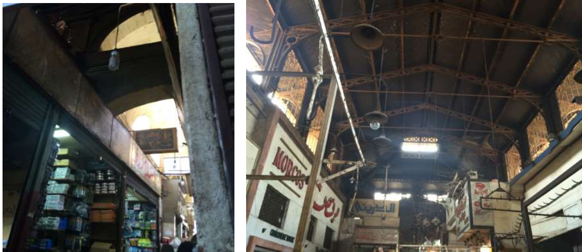
Figure 5. The Clerestory to provide natural daylight and ventilation inside the building: Left, the secondary alleyways; Right, the main Alleyway trusses and side openings (Source: author's collection).
