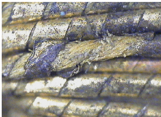
Fig. 2. An image of the corroded copper threads using the reflected optical microscope. (For interpretation of the references to color in this figure legend, the reader is referred to the web version of the article.)
