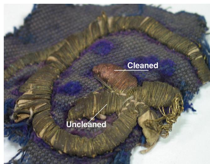
Fig. 6. An optical microscopy image shows the surface appearance of the tested metal threads after the laser cleaning. (For interpretation of the references to color in this figure legend, the reader is referred to the web version of the article.)
