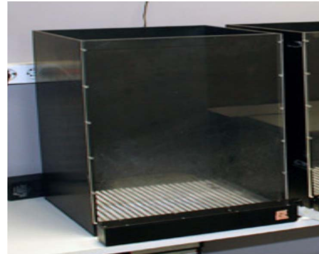
Foot shock-induced aggression apparatus
