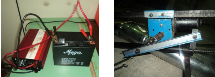
Fig. (8) Power unit and reciprocating mechanism of the developed machine.
