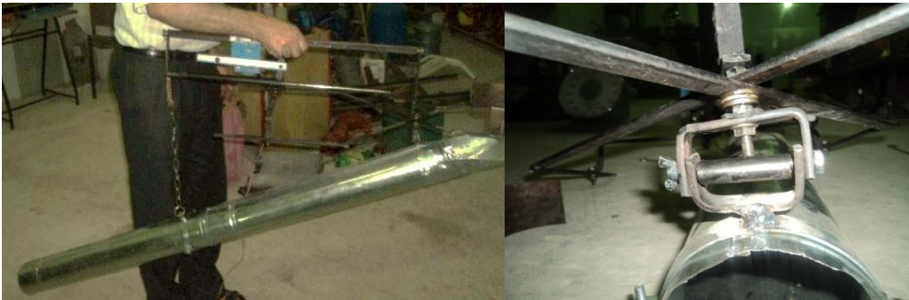
Fig. (7): Cylindrical transport device of the developed machine.
