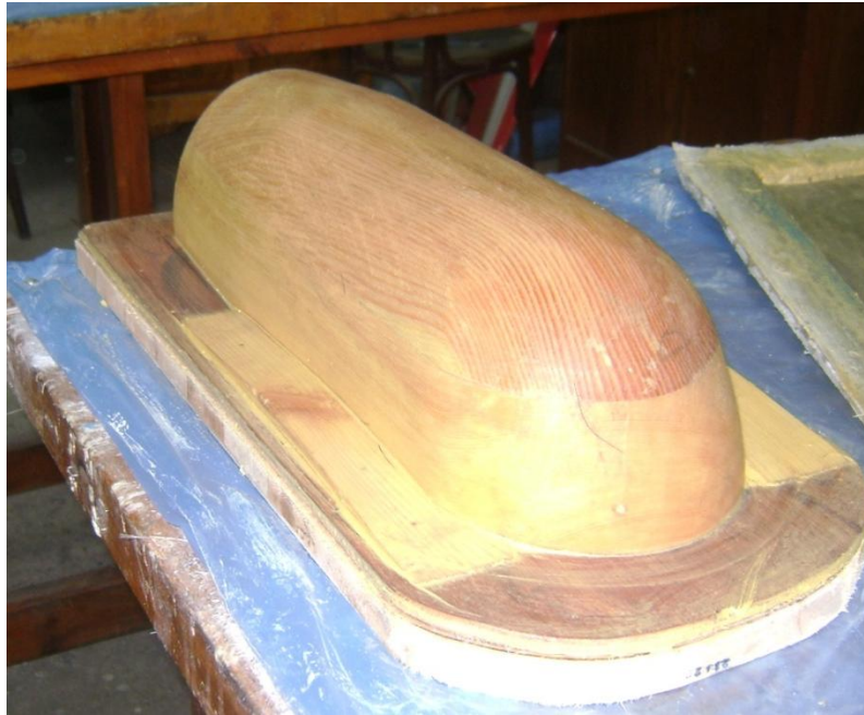
Figure 140: Fuselage master mold
