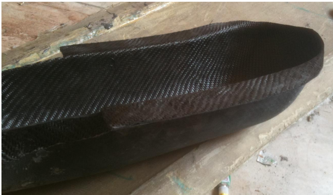
Figure 143: Fuselage body-2 "after trimming"
