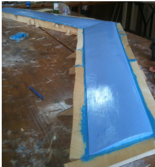
Figure 127: Klean Klay filling
