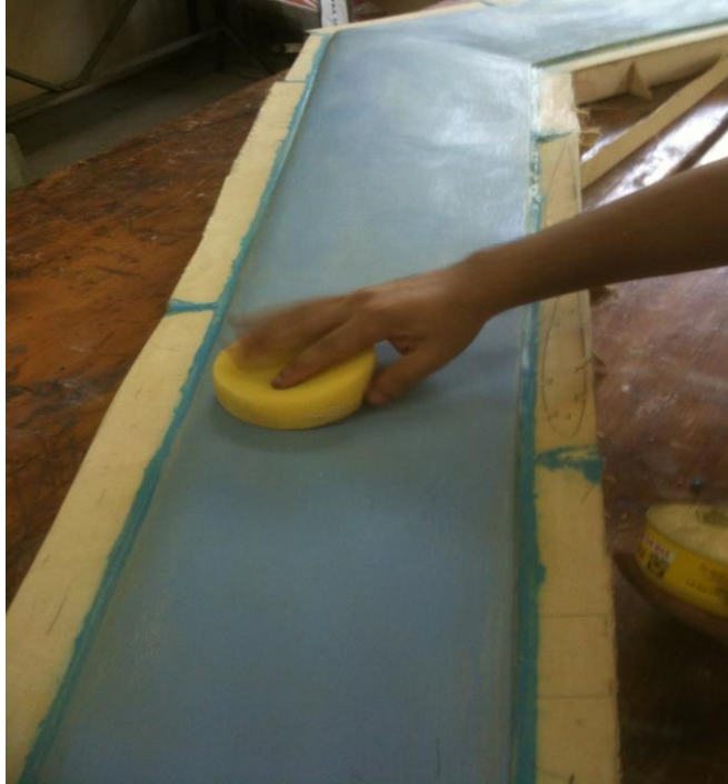
Figure 128: Master mold isolation
