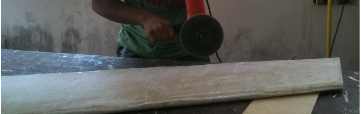
Figure 124: Master mold sanding
