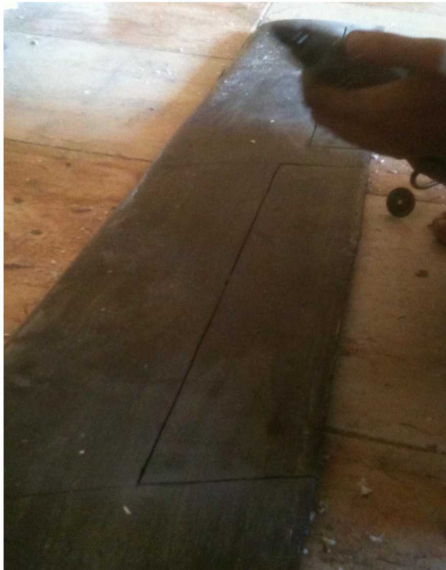
Figure 135: Cutting Control Surfaces
