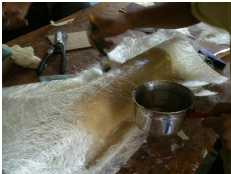
Figure 141: Female mold making
