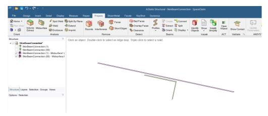
There is a problem in this configuration that the two surfaces should be connected together. To do so, we will use the move option
