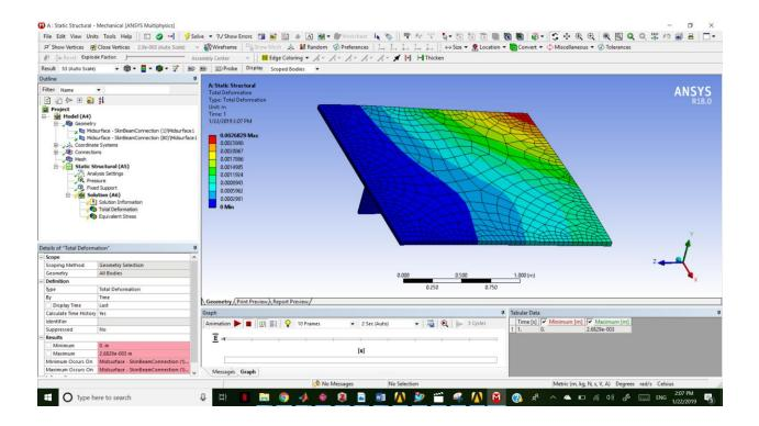
The correct method is to leave the distance between the two bodies as it is and define contacts manually in Ansys model.
