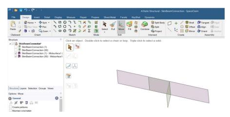
Open ansys model to excute a finite element model for the body. Notice that Ansys by default will define
