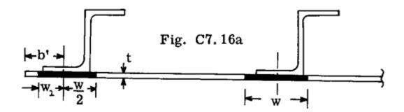
If the stringers and skins have different material properties. We multiply the effective width equation by a correction factor  $\frac{F_{sh}}{F_{st}}$ .
