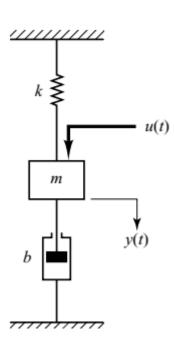
This system is of second order. This means that the system involves two integrators. Let us define state variables  $x_1(t)$  and  $x_2(t)$  as
