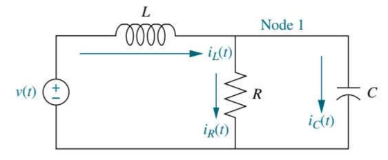
Apply network theory, such as Kirchhoff's voltage and current laws, to obtain  $i_C$  and  $v_L$  in terms of the state variables,  $v_C$  and  $i_L$ . At Node 1,
