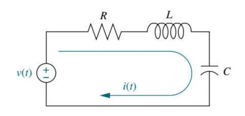
Which represents a second order D.E. that can be transformed into two first order D.E's with two state variables
