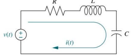
This equation is known as the <u>output equation</u>; we say that  $v_L(t)$  is a linear combination of the state variables, q(t) and i(t), and the input, v(t).
