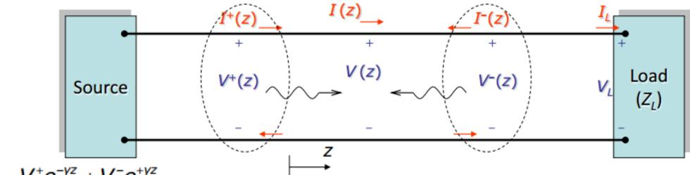
$$V(z) = V_0^+ e^{-\gamma z} + V_0^- e^{+\gamma z}$$
