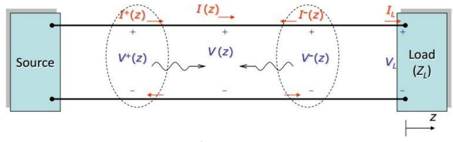
$$V(z) = V_0^+ \left( e^{-\gamma z} + \Gamma_L e^{+\gamma z} \right)$$
