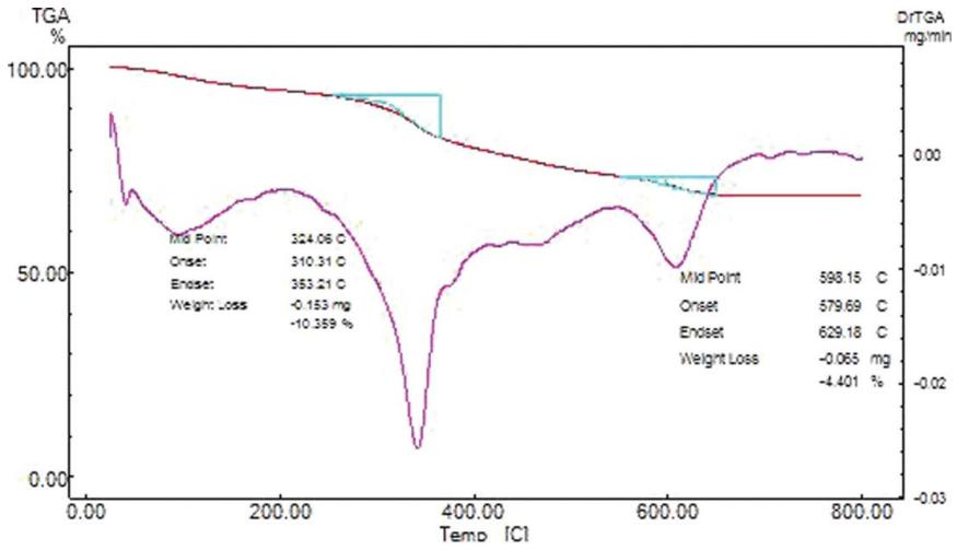
Figure 2. DTA-TGA analysis of the yttria precursor.
