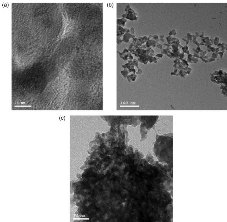
Figure 4. (a) The TEM image shows crystallinity of the yttria nanoparticles annealed at 450 °C. (b) The TEM image shows morphological shape of the yttria nanoparticles. (c) The TEM image shows high degree of agglomeration of the yttria nanoparticles.
