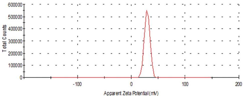
Figure 6. Pattern of Zetapotential of yttria nanoparticles.
