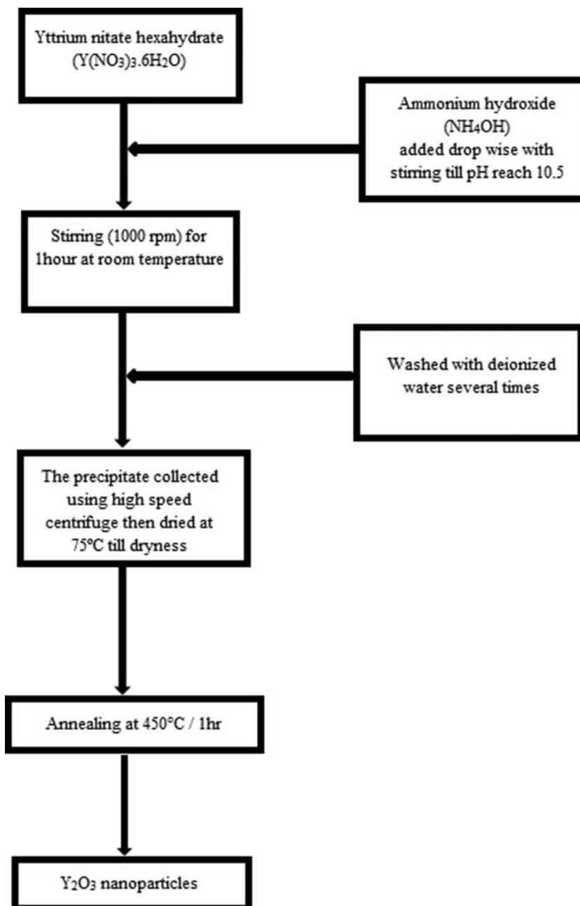
Figure 1. Synthesis of Y<sub>2</sub>O<sub>3</sub> nanoparticles by chemical precipitation.
