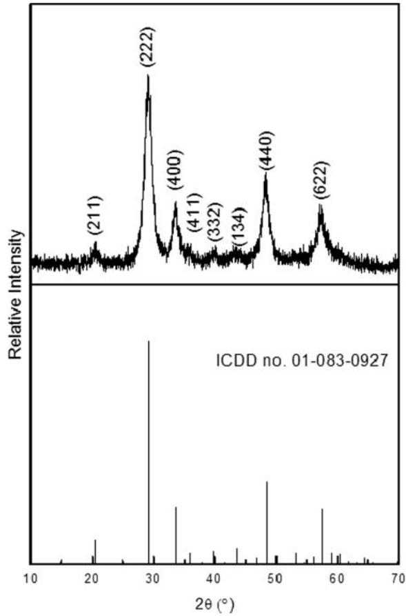
Figure 3. XRD pattern of yttria nanoparticles (YNPs)
