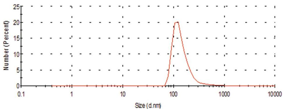
Figure 5. Pattern of DLS of yttria nanoparticles.
