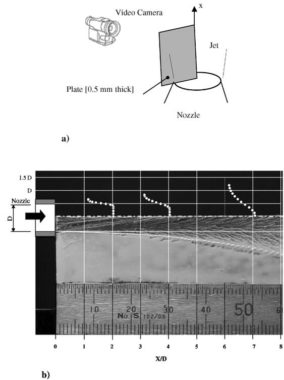
Fig. 11. Oil flow visualization: a) Experimental arrangement for oil flow visualization; b) Jet boundary visualized by oil flow.
