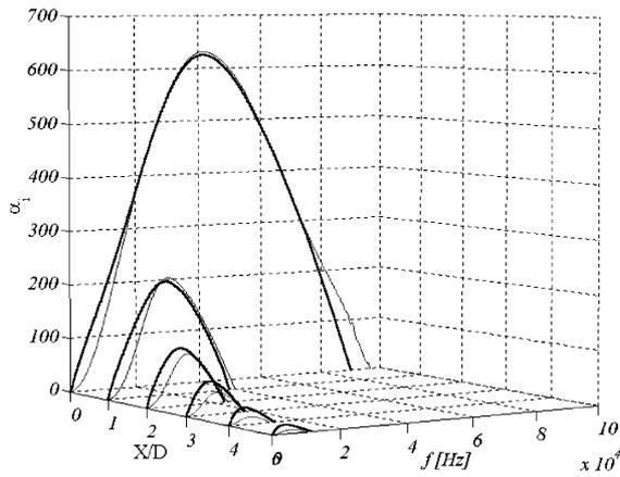
Fig. 10. Dimensional stability curves at different axial locations for “—” axisymmetric ( $n = 0$ ); “- - -” asymmetric ( $n = 1$ ) disturbance modes.
