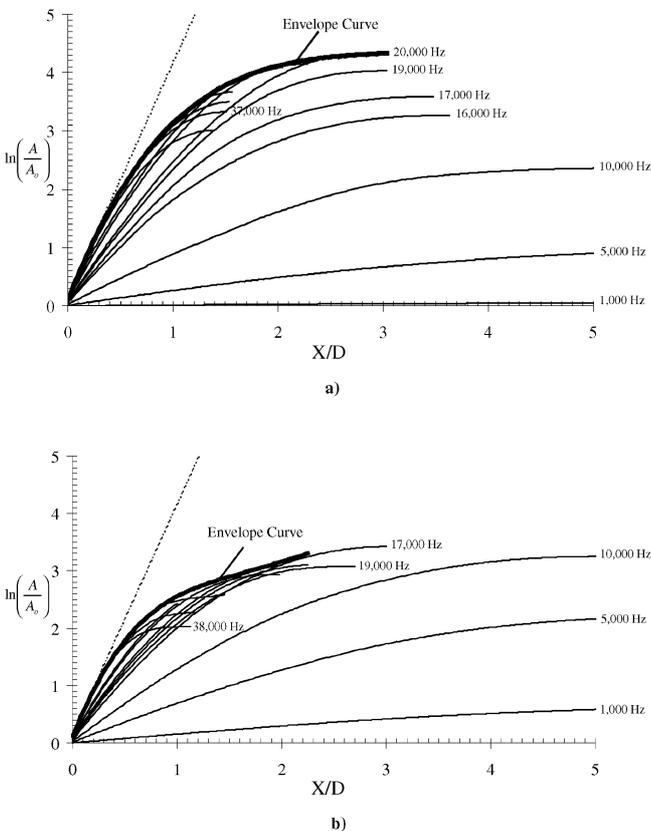
Fig. 15. Envelope curve for instability growth: a) Axisymmetric disturbance modes ( $n = 0$ ); b) Asymmetric disturbance mode ( $n = 1$ ).
