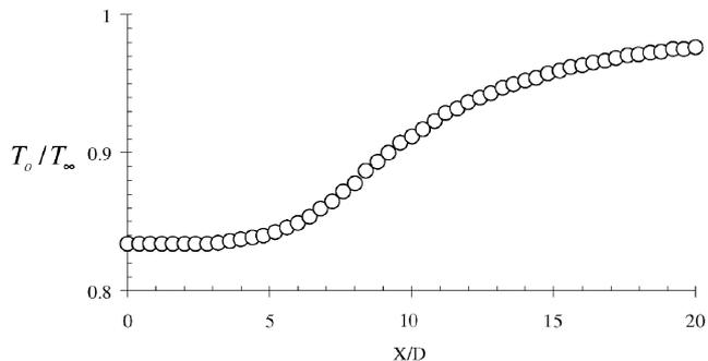
Fig. 3. Jet centerline temperature distribution normalized by ambient temperature.
