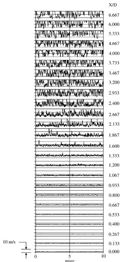
Fig. 14. Velocity fluctuations measured by hot wire at different axial locations.
