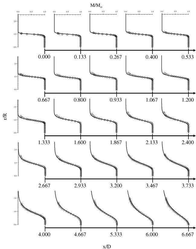
Fig. 4. Radial Mach number distributions at different axial locations.  $\circ$ : experimental data; —: hyperbolic - tangent velocity profile.
