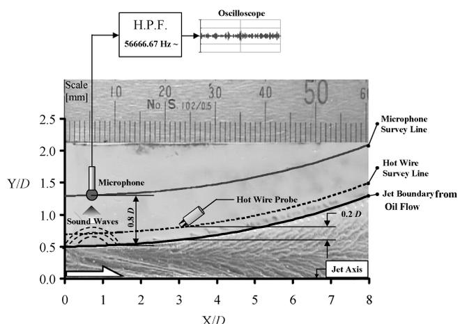
Fig. 12. Experimental setup for transition detection.
