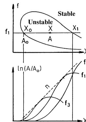
Fig. 1. Principle of the  $e^N$  method [D. Arnal<sup>2)</sup>].
