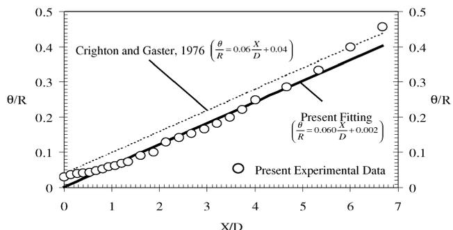
Fig. 5. Axial variation of the ratio of momentum thickness to jet radius,  $\theta/R$ .
