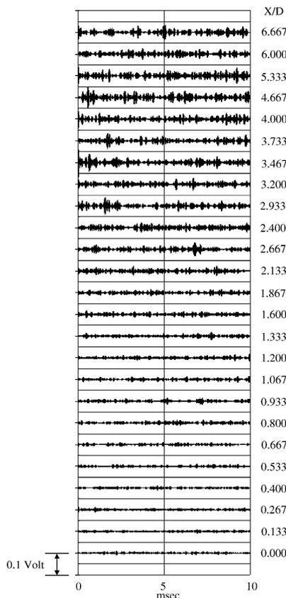
Fig. 13. HPF microphone signals at different axial locations.
