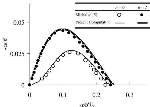
Fig. 7. Jet linear stability test case of the hyperbolic-tangent velocity profile (Eq. 10) with  $R/\theta = 6.25$ ,  $M_0 = 1.2$  and  $T_0/T_\infty = 1$  (isothermal flow).
