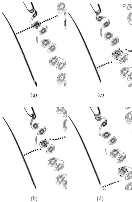
Fig. 9. Particles movement and vortex motion (entropy contours).
