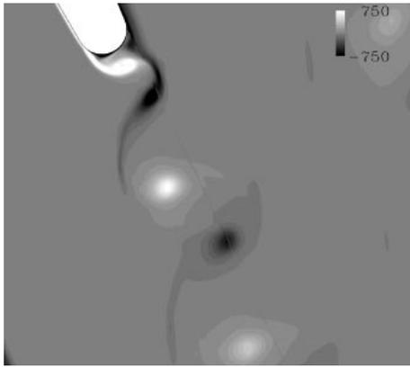
Fig. 8. Contours of instantaneous non-dimensional vorticity.
