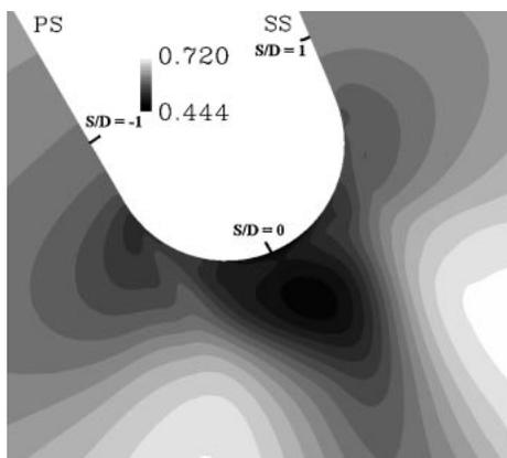
Fig. 5. Contours of time-averaged non-dimensional pressure near trailing edge; PS: pressure side; SS: suction side.
