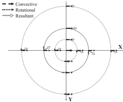
Fig. 11. Superposition of velocity.
