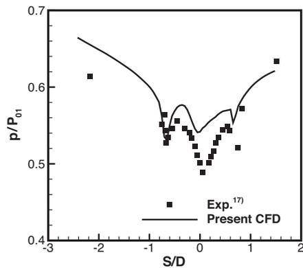
Fig. 4. Distributions of time-average pressure along trailing edge.
