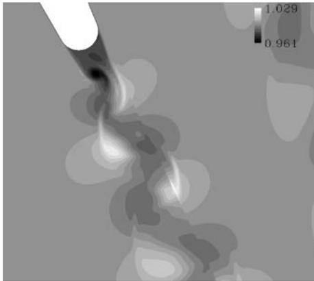
Fig. 13. Instantaneous non-dimensional total temperature contours at  $M_{2,is} = 0.4$ .
