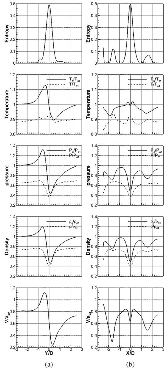
Fig. 12. Flow properties along: (a) transverse direction; (b) tangential direction.
