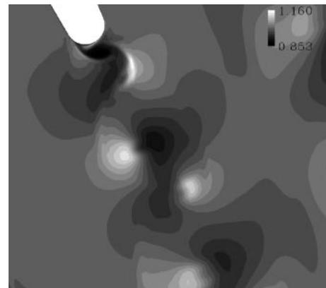
Fig. 7. Instantaneous non-dimensional total temperature contours.
