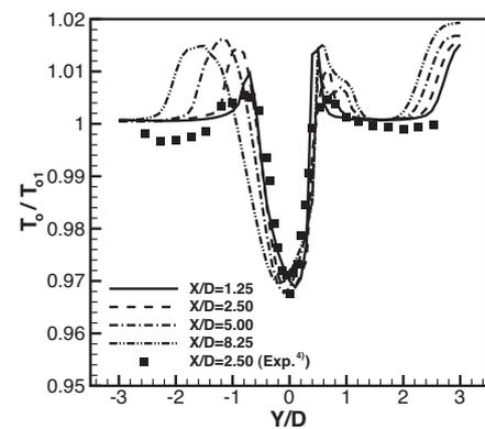
Fig. 15. Time-average total temperature distribution in wake.
