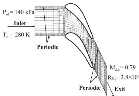
Fig. 2. Computational grid and boundary conditions.
