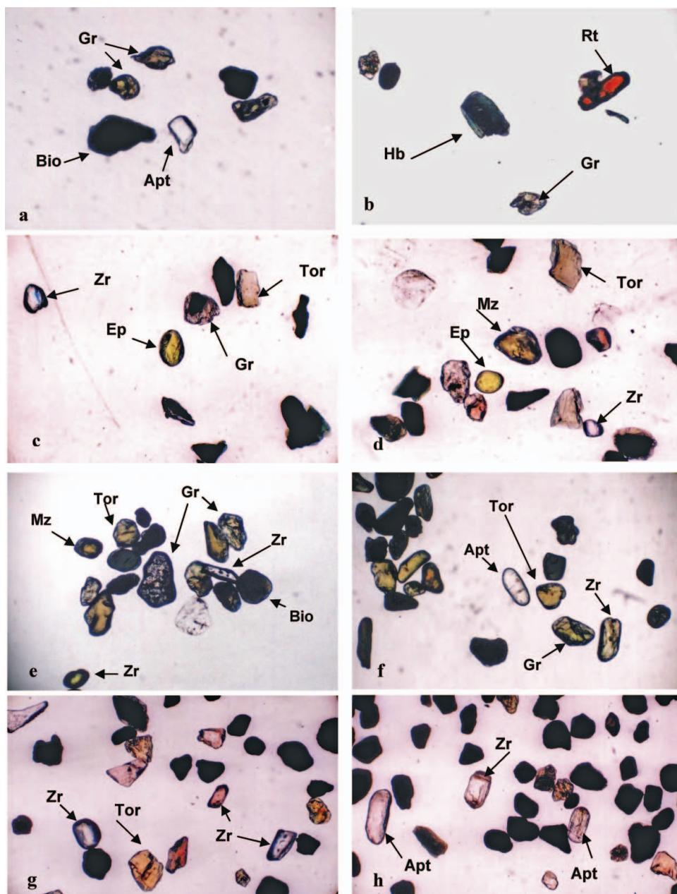
**Figure 6** Photomicrograph showing some heavy mineral associations in the soil of the study black sand sites. (a & b) sand mounds in Abu Khashaba, (c & d) coastal sand plain in Abu Khashaba and (e & f) coastal sand dune in Baltim, and (g & h) minerals in the control soil. Gr = Garnet; Ep = Epidote; Rt = Rutile; Hb = Hornblende; Apt = Apatite; Bio = Biotite; Zr = Zircon; Tor = Tourmaline; and Mz = Monazite. (Figure available in color online.)
