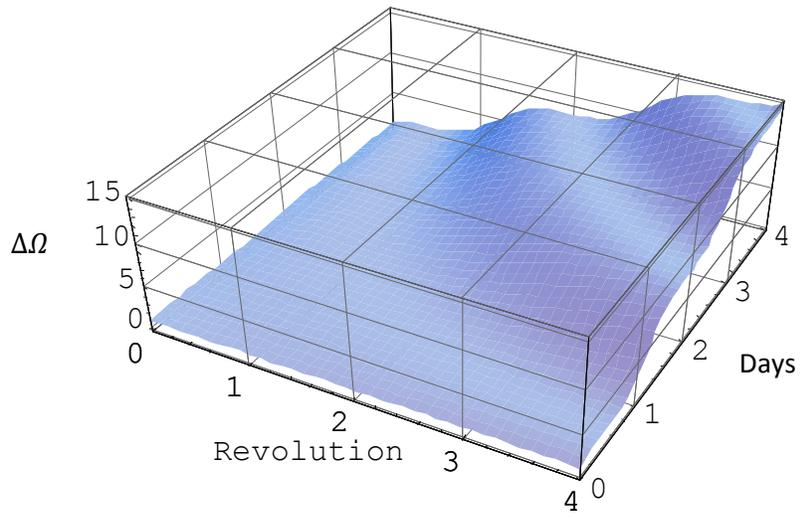
Figure 2. The variations of the orbital plane by angle  $\Omega$  for polar orbit
