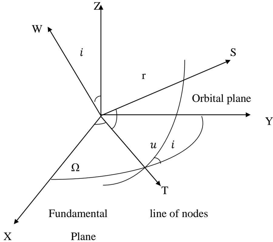
**Fig. 1** The disturbing force of gravitational waves in (S, T, W) directions
