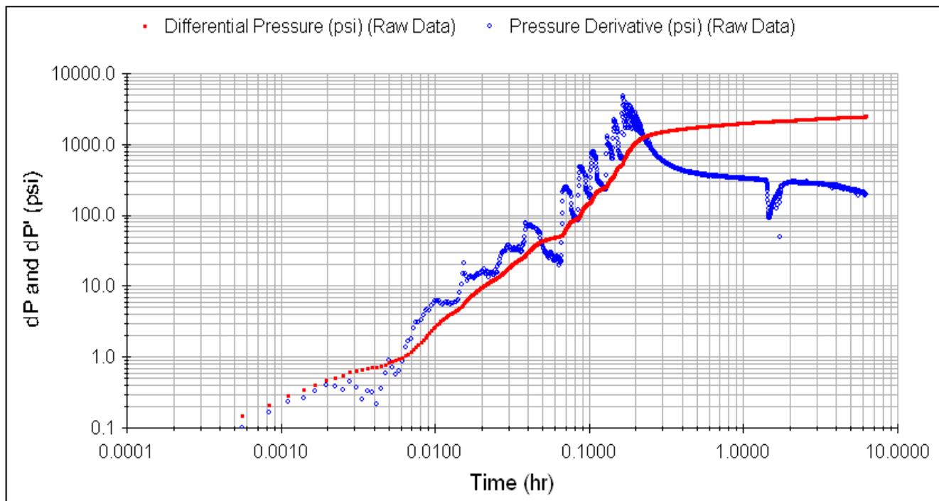
**Fig. 4 Log-Log plot of observed pressure change and it's logarithmic during injection fall-off test in West Coast Africa Field case**
