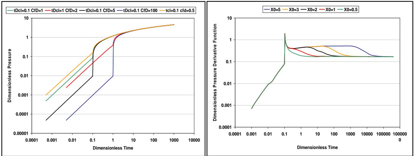
**Fig.1 a) Computed pressure change  $\Delta p_D$  after shut-in for various fracture compliance and fracture closure time. Dual mobility Zones; mobility ratio=0.33 b) Computed Logarithmic derivative of the pressure change after shut-in for various mobility interface positions. Dual mobility Zones;  $C_{fd} = 1$ ;  $t_{Dcl} = 0.1$ ; mobility ratio=0.33**
