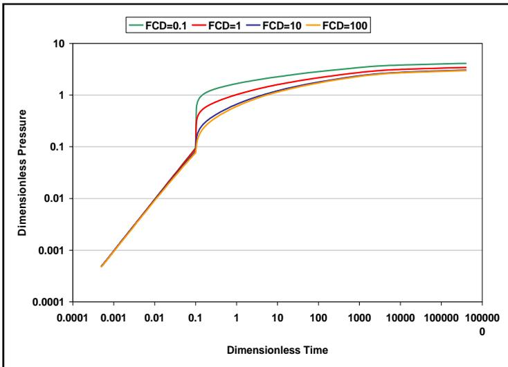
**Fig.2 a) Computed pressure change  $\Delta p_D$  after shut-in for various fracture conductivity. Dual mobility Zones; fracture closure time=0.1, mobility ratio=0.33, fracture compliance=1, Skin=0**
