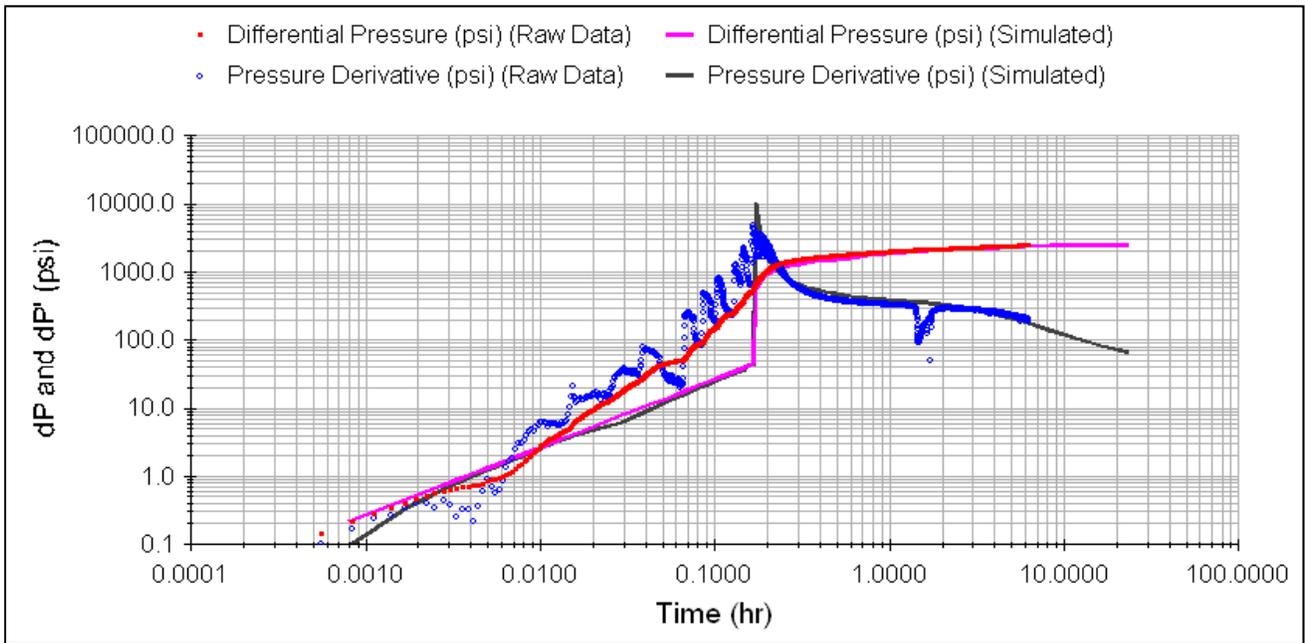
Fig. 5 Log-Log plot of observed pressure change and its logarithmic during injection fall-off test in West Coast Africa Field Case (A match with the infinite conductivity model)
