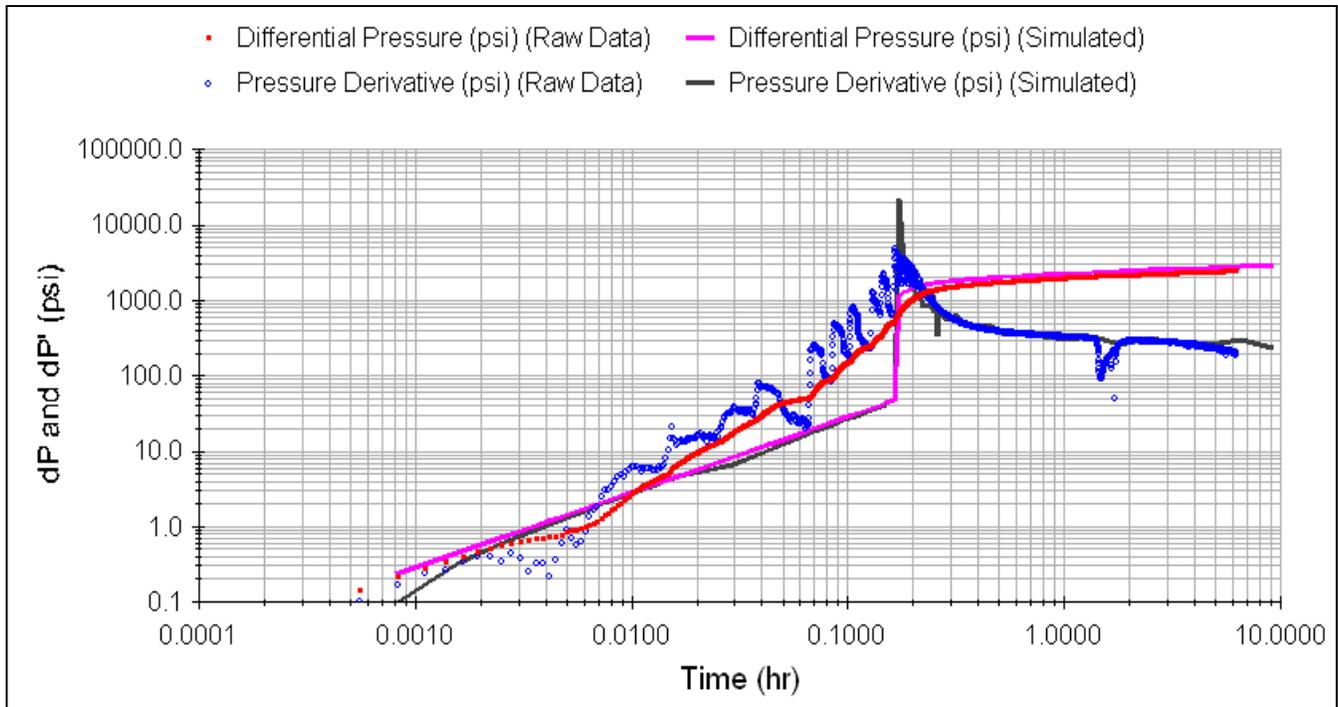
Fig. 7 Log-Log plot of observed pressure change and its logarithmic during injection fall-off test in West Coast Africa Field Case (A match with the finite conductivity model with dual mobility zones and fracture face skin)
