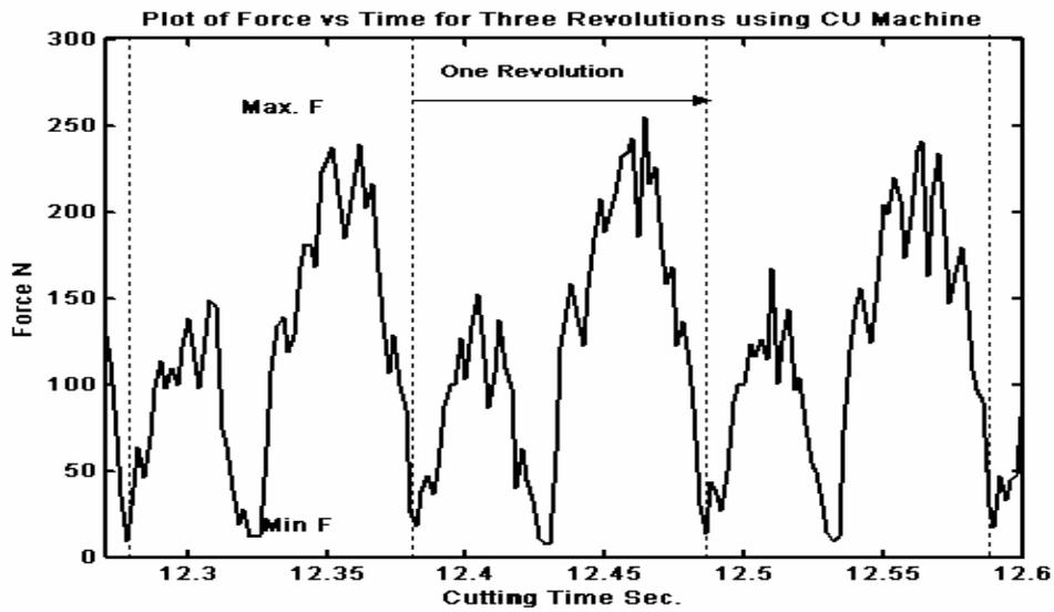
Figure 2. Force vs. Time for Three Revolutions.
