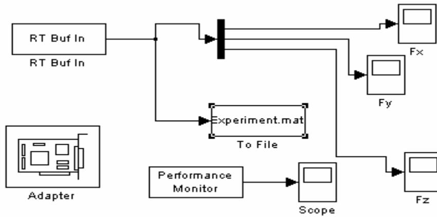
Figure 4. SIMULINK Simulation Model Used to Measure the Cutting Forces.
