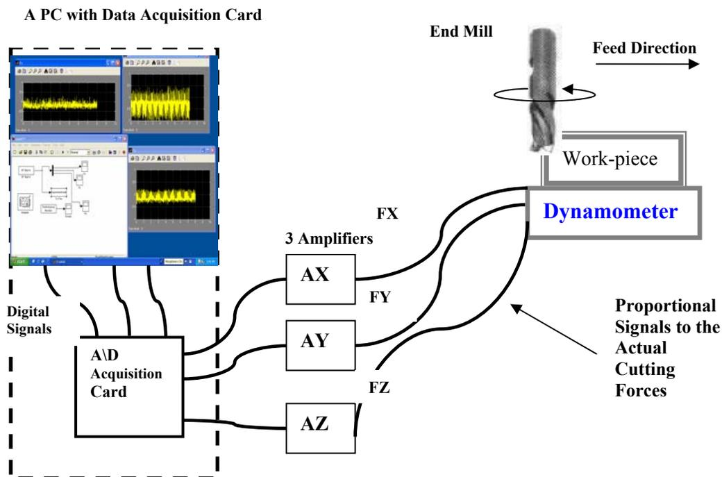
Figure 5. The Experimental Setup.
