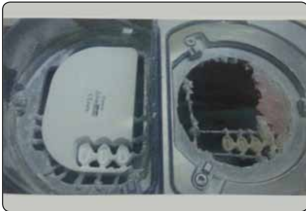
Fig. (4) Milling of zirconia prattau (Group II)
