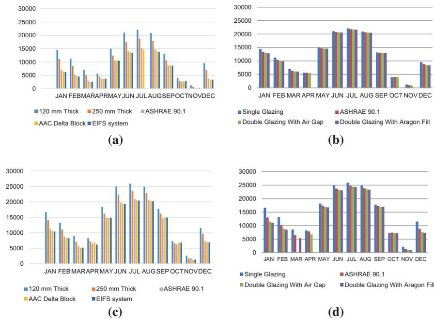
**Fig. 5** Monthly energy consumption for the different retrofit façade retrofit schemes. (a) Opaque in a regular window façade. (b) Translucent in a regular window façade. (c) Opaque in double-skin façade. (d) Translucent in double-skin façade
