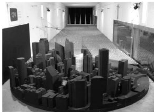
Fig. 2 Schematic and internal view of wind tunnel test
