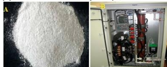
Fig.1: Micronized clinoptilolite zeolite powder. B: Envirolite reactor: [(HClO, ClO 2 , HClO 3 , HClO 4 , H 2 O 2 , O 2 , ClO - , ClO 2 - , ClO 3 - , O - , HO 2 - , OH - - working substances), pH 2.5-3.5, ORP>1150mV, active chlorine ~500mg/l.
