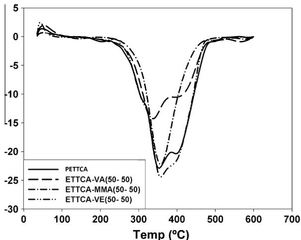
Fig. 6. Differential thermogravimetric analysis (DTGA) of ETTCA-VA, ETTCA-VE and ETTCA-MMA copolymers.
