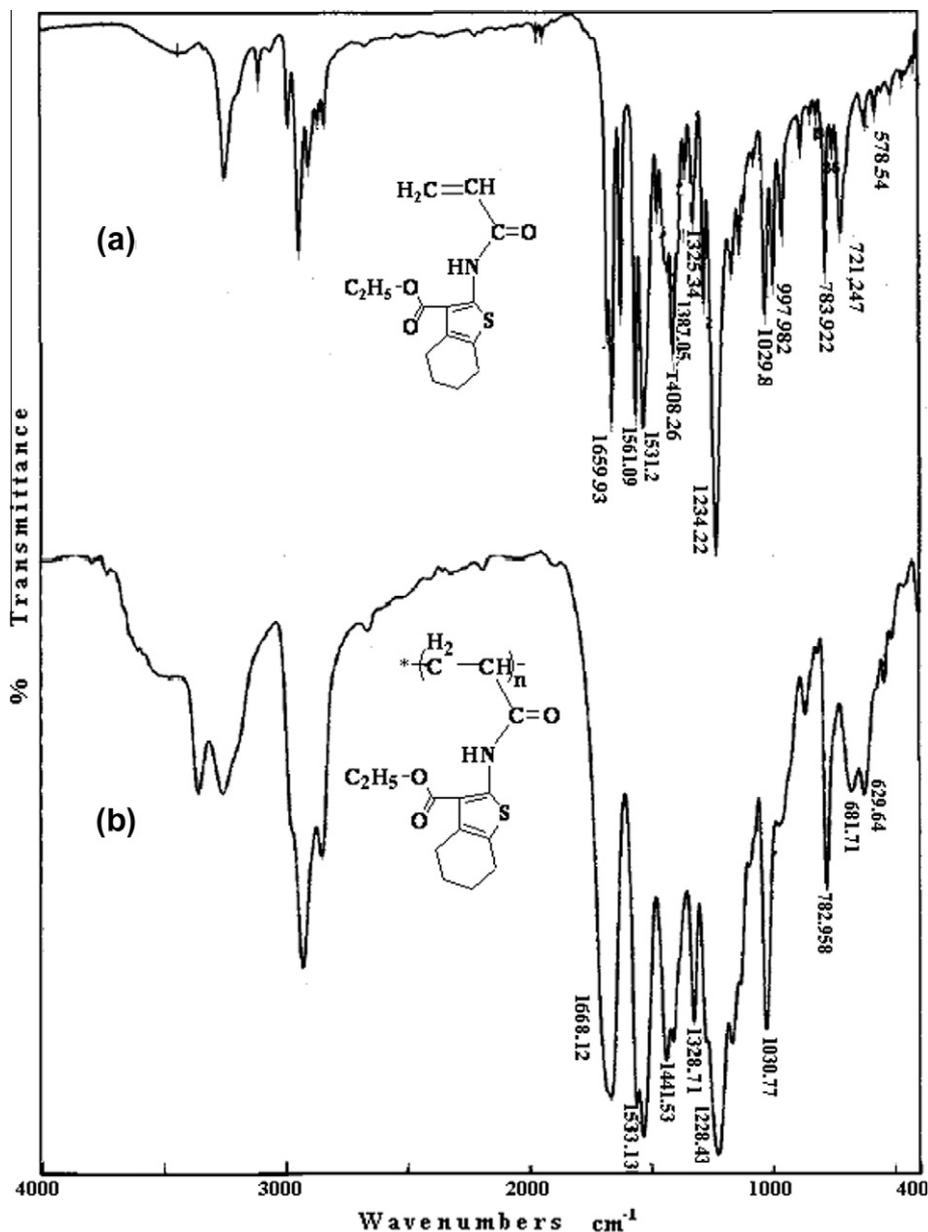
Fig. 1. FTIR spectra for the monomer ETCA and of its polymer.
