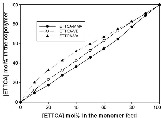
**Fig. 4.** Copolymer composition curves for the three systems ETTCA with VA, MMA and VE.
