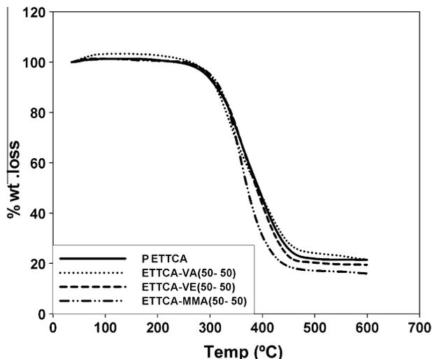
Fig. 5. Thermogravimetric analysis of ETTCA-VA, ETTCA-VE and ETTCA-MMA copolymers.
