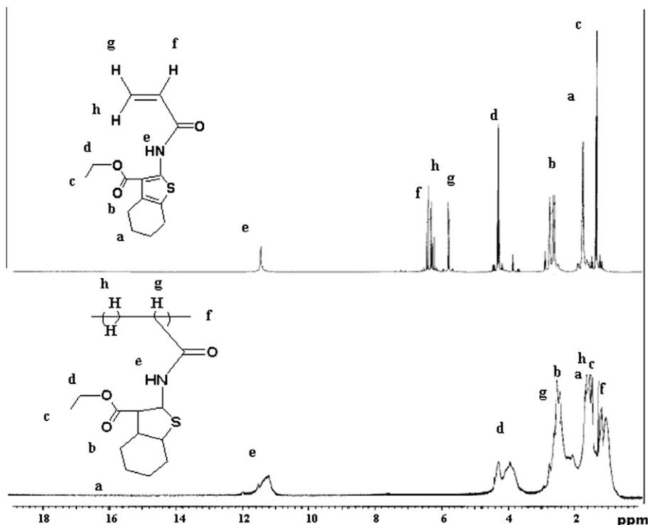
Fig. 2. <sup>1</sup>H NMR spectra for the monomer ETTCA and of its polymer.
