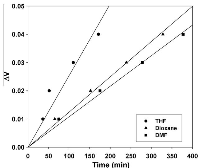
**Fig. 3.** The relation between the volume contraction  $\Delta V$  of ETTCA polymerization and time in different solvents [ETTCA] = 0.2 M [AIBN] =  $8.1 \times 10^{-4}$  M and at 65 °C.
