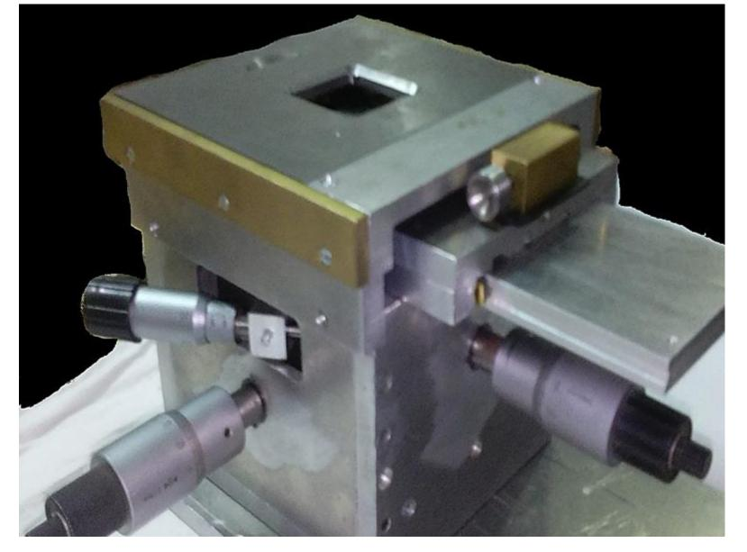
The Mask Aligner, for Uv exposure I use Uv Led Array (15x15) on a Pcb connected in parallel, I use a Usb digital microscope after having replaced its white Led with yellow/orange/red Led light source.
